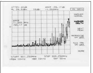
The following 2 plots shows that there are no emissions within 20 dB of the inband signal in any 100 kHz band all the way to the  $10^{th}$  harmonic.
