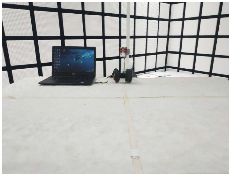
Radiated spurious emission Test Setup-3(Above 1GHz)
