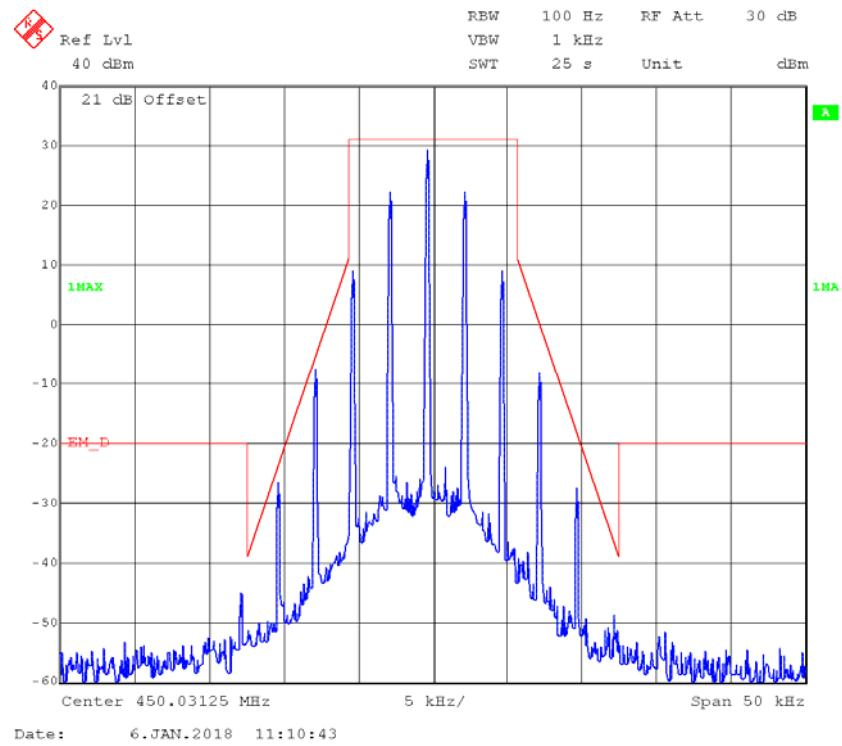
**FM,25kHz,High Power - Frequency 450.03125 MHz: 99% Occupied & 26 dB Bandwidth**
