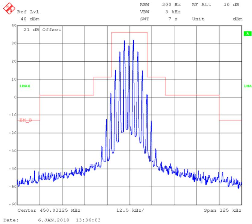
**FM,25kHz,Low Power - Frequency 450.03125 MHz: 99% Occupied & 26 dB Bandwidth**
