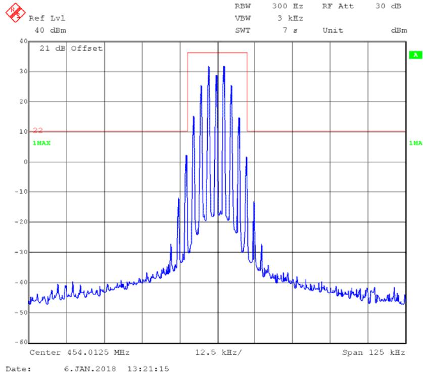
**FM,25kHz,Low Power - Frequency 454.0125 MHz: 99% Occupied & 26 dB Bandwidth**
