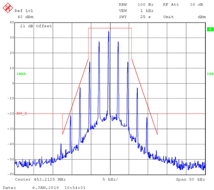
**FM,12.5kHz,Low Power - Frequency 453.2125 MHz: 99% Occupied & 26 dB Bandwidth**
