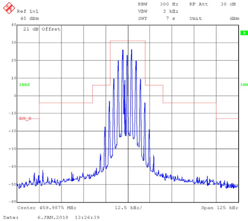
**Part 74****FM,12.5kHz,High Power - Frequency 450.03125 MHz: 99% Occupied & 26 dB Bandwidth**
