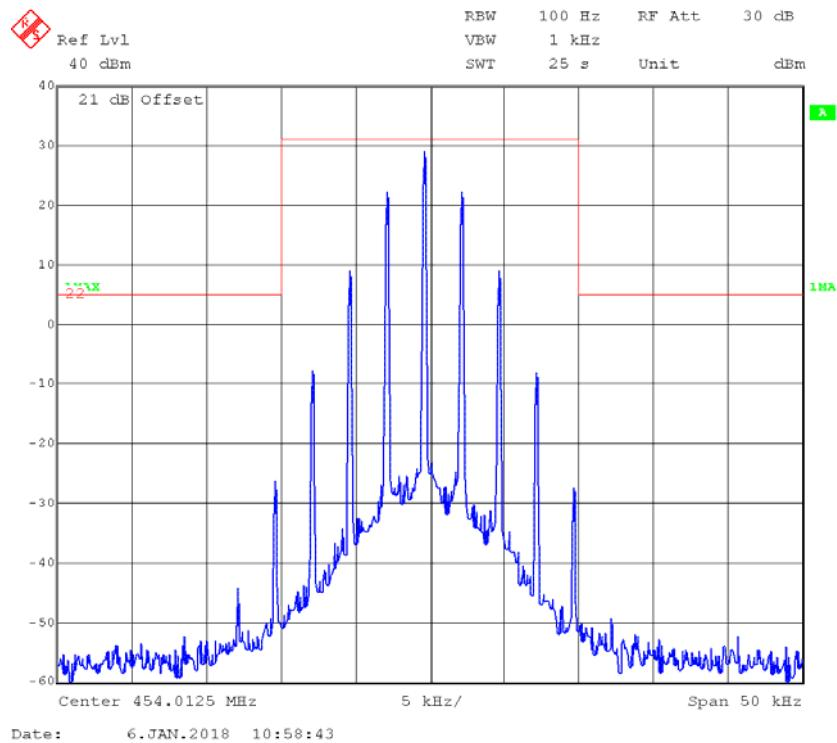
**FM,25kHz,High Power - Frequency 454.0125 MHz: 99% Occupied & 26 dB Bandwidth**
