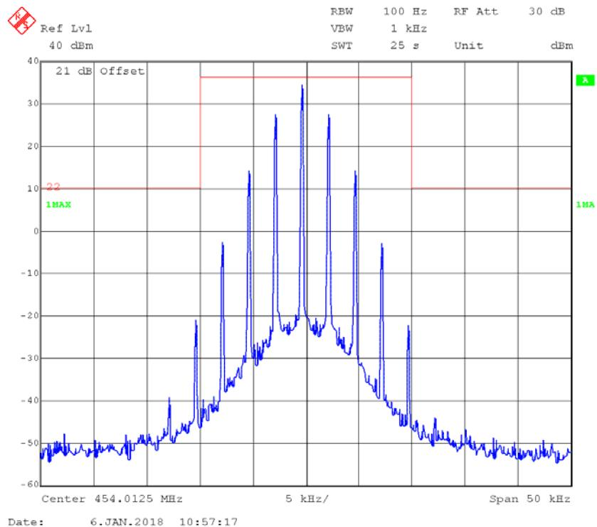
**FM,12.5kHz,Low Power - Frequency 454.0125 MHz: 99% Occupied & 26 dB Bandwidth**
