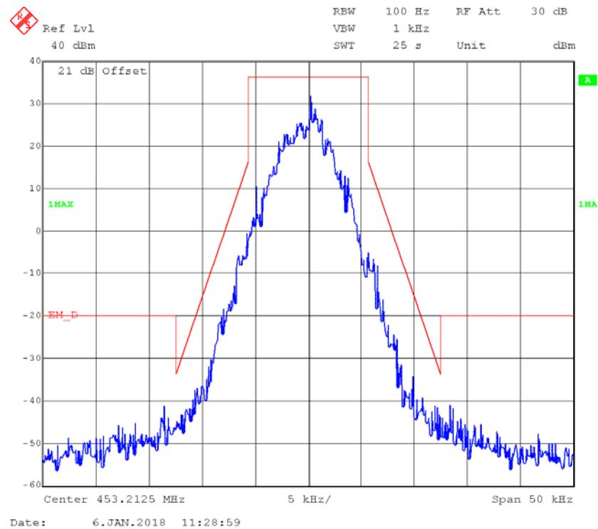
**4FSK,12.5kHz,Low Power - Frequency 453.2125 MHz: 99% Occupied & 26 dB Bandwidth**
