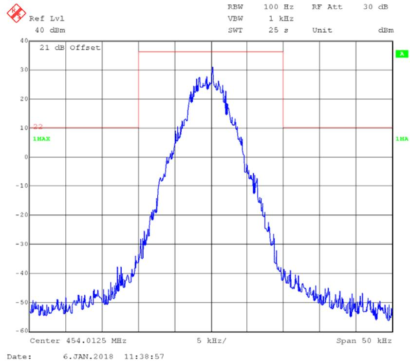
**4FSK,12.5kHz,Low Power - Frequency 454.0125 MHz: 99% Occupied & 26 dB Bandwidth**
