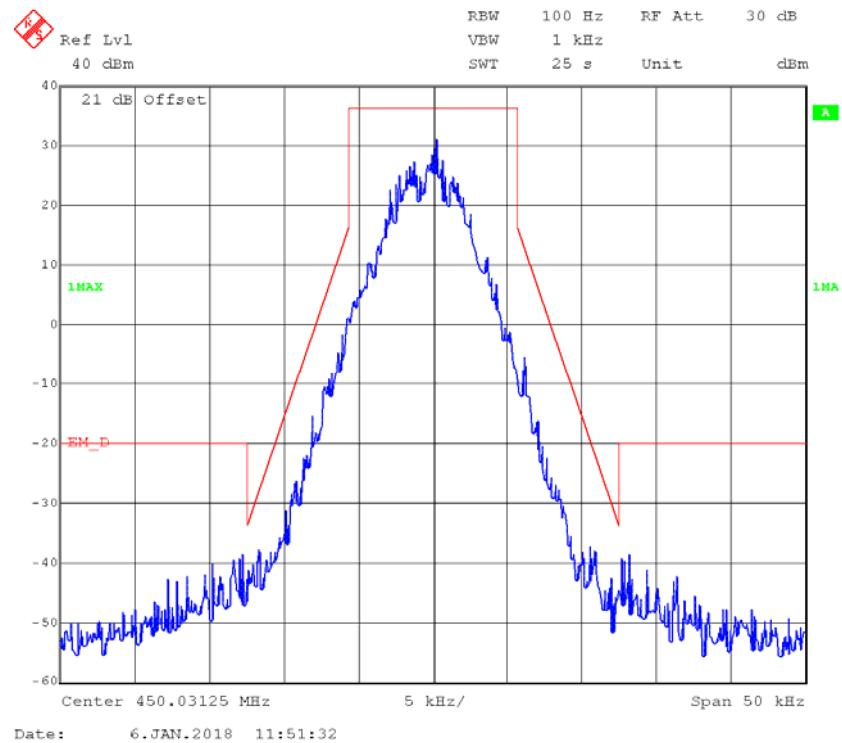
**4FSK,12.5kHz,Low Power - Frequency 450.03125 MHz: 99% Occupied & 26 dB Bandwidth**
