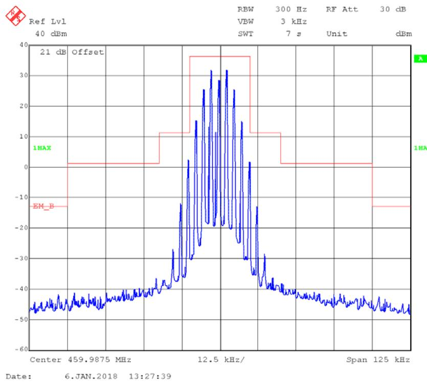
**FM,25kHz,Low Power - Frequency 459.9875 MHz MHz: 99% Occupied & 26 dB Bandwidth**
