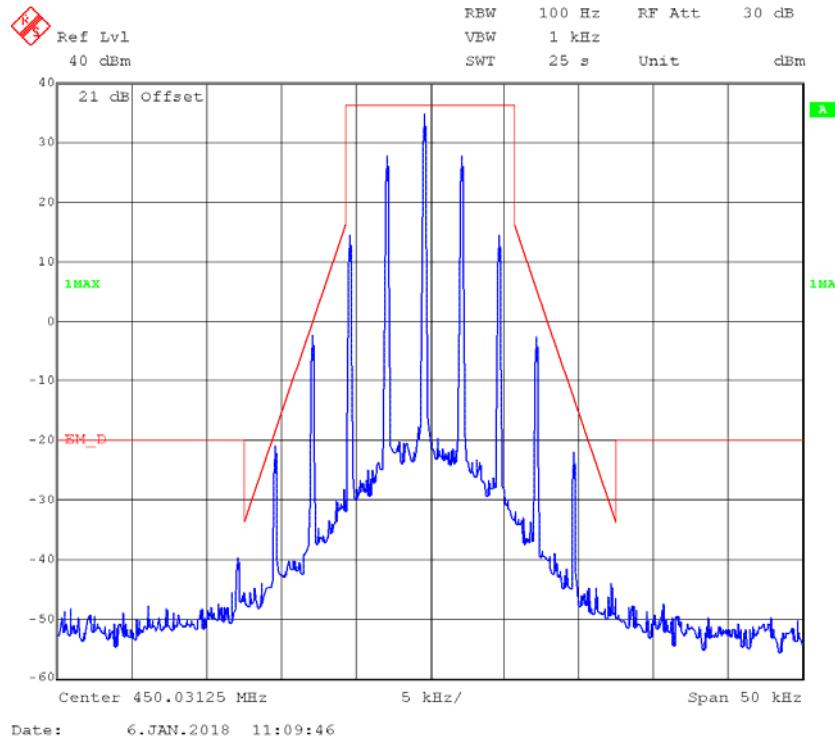
**FM,12.5kHz,Low Power - Frequency 450.03125 MHz: 99% Occupied & 26 dB Bandwidth**
