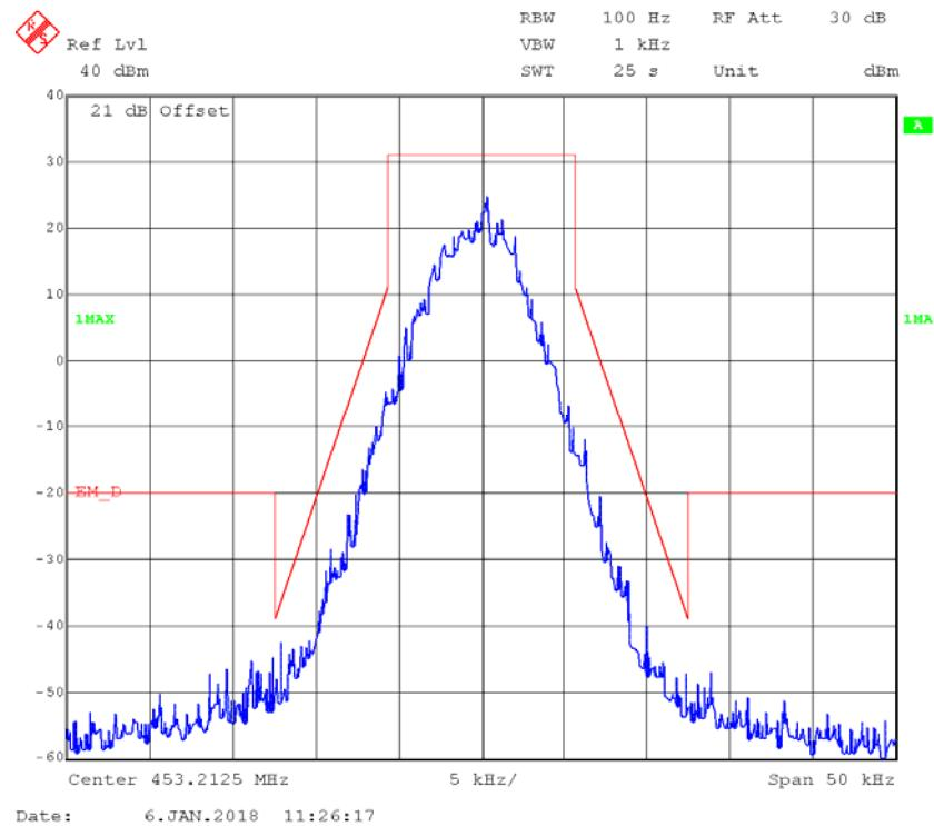
**Part 80:****FM,25kHz,High Power - Frequency 459.9875 MHz MHz: 99% Occupied & 26 dB Bandwidth**
