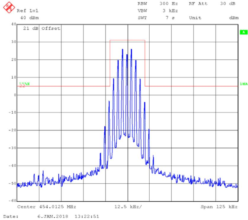
**4FSK,12.5kHz,High Power - Frequency 454.0125 MHz: 99% Occupied & 26 dB Bandwidth**
