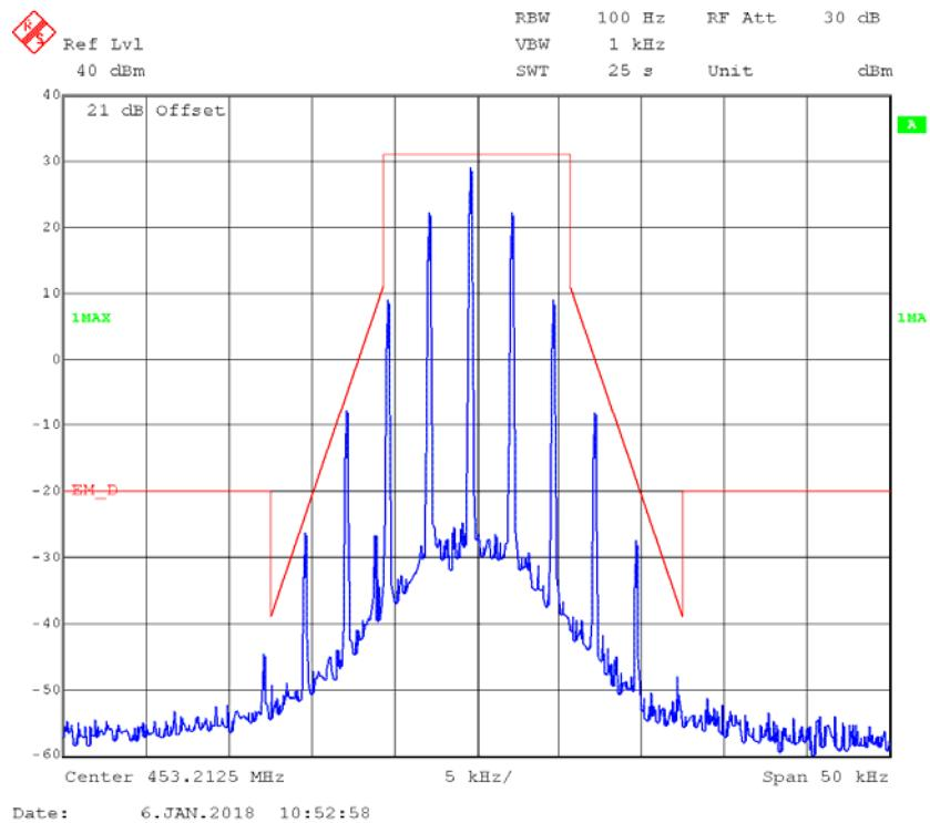
**4FSK,12.5kHz,High Power - Frequency 453.2125 MHz: 99% Occupied & 26 dB Bandwidth**
