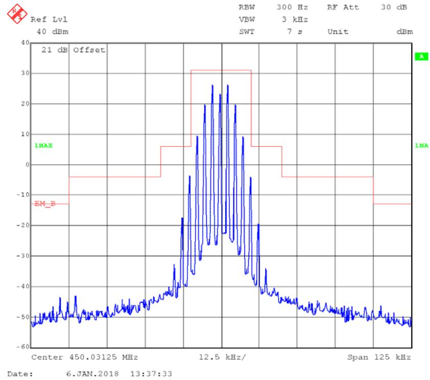
**4FSK,12.5kHz,High Power - Frequency 450.03125 MHz: 99% Occupied & 26 dB Bandwidth**
