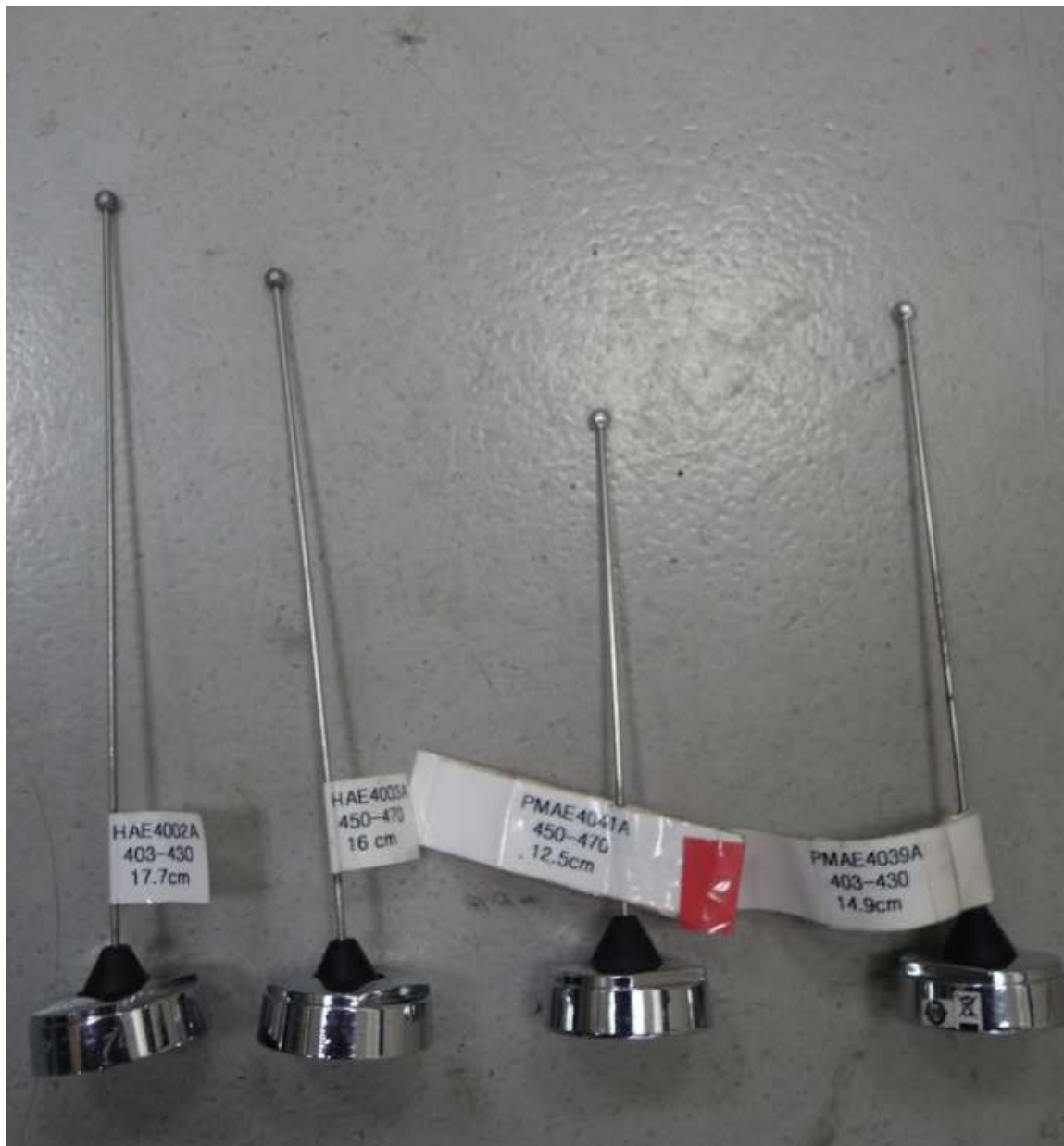
UHF Antenna kit numbers, from left to right HAE4002A, HAE4003, PMAE4039A, PMAE4041A
