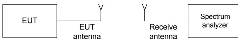
Figure 7.2.1 Carrier frequency separation test setup
