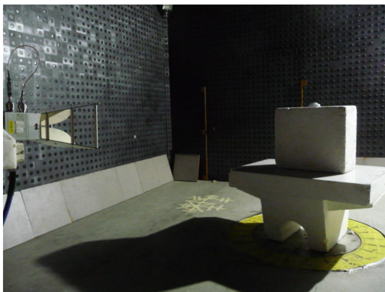
Photograph 8.1.2 Setup for radiated emission measurements above 1 GHz
