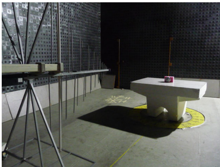
Photograph 8.1.2 Setup for radiated emission measurements above 1 GHz
