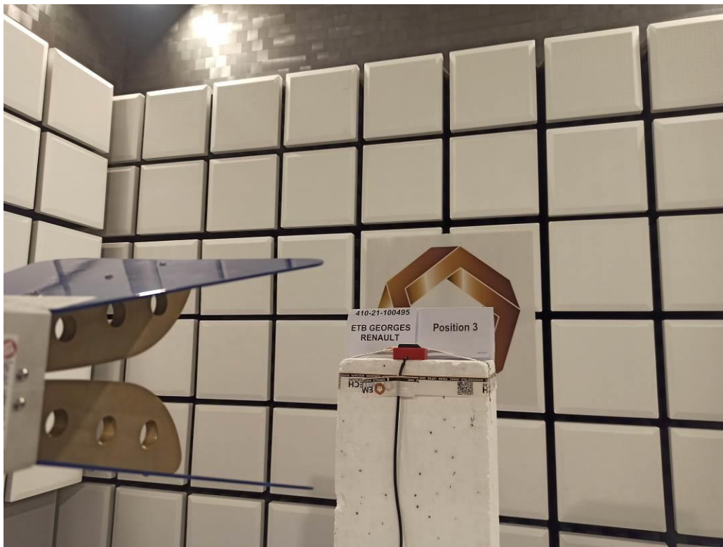
TEST SETUP PHOTO(S) - 960MHz TO 18GHz
