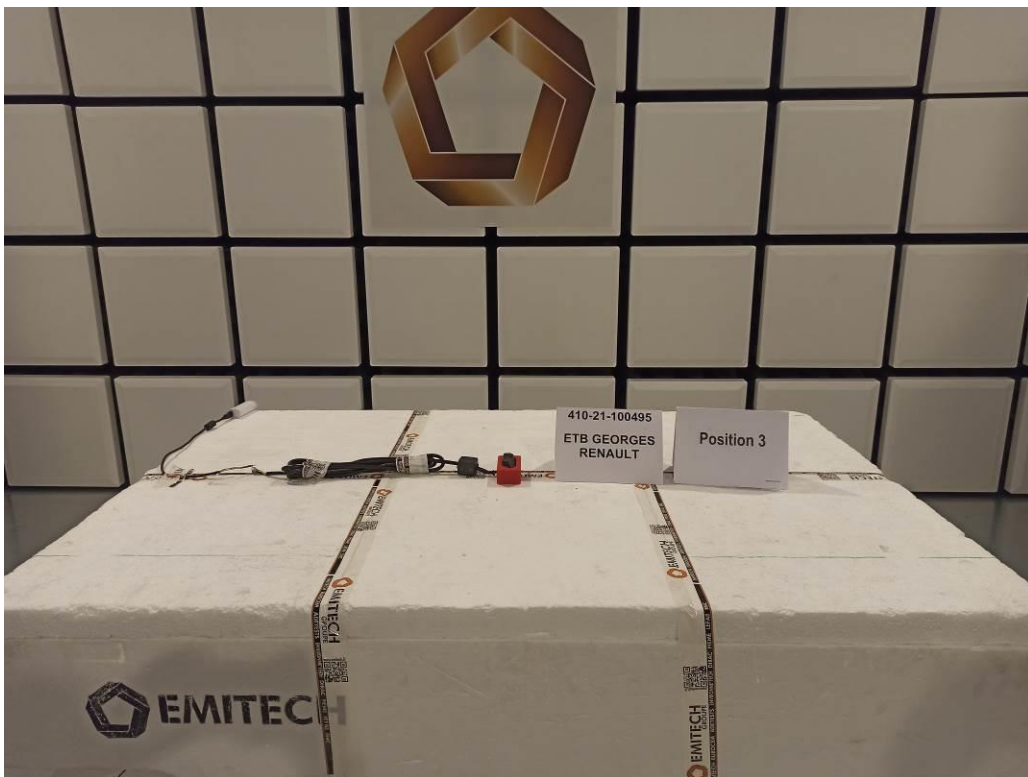
TEST SETUP PHOTO(S) - RADIATED MEASUREMENT <960MHz / POSITION 3
