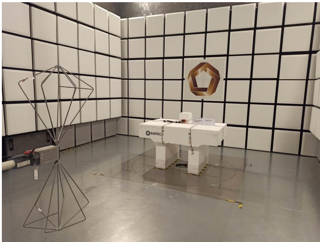
TEST SETUP PHOTO(S) - 30MHZ TO 200MHZ
