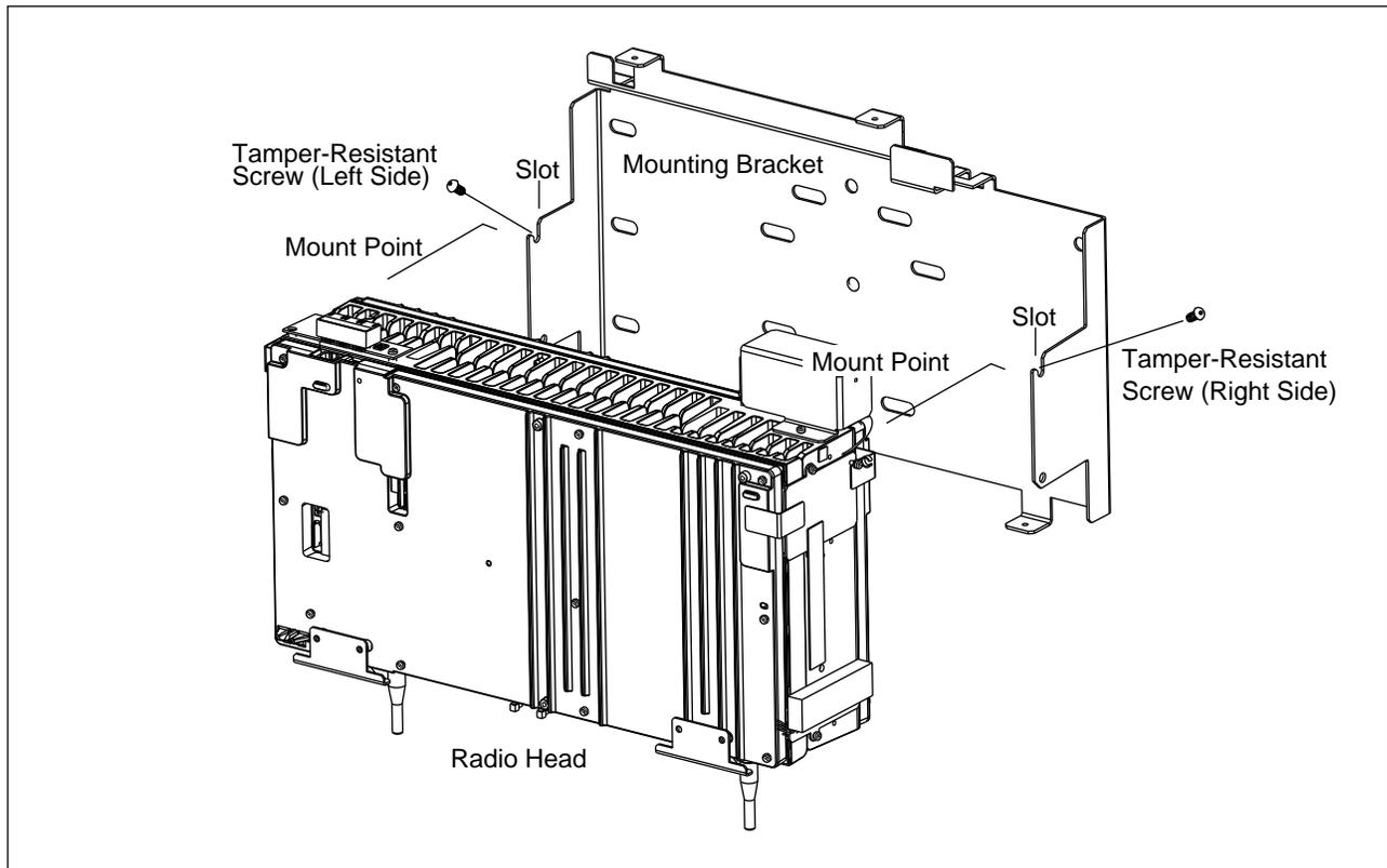
Figure 6-18. Removing Radio Head from Mounting Bracket
