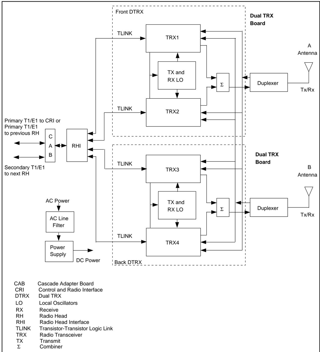
Figure A-2. Radio Head Transmission Path
