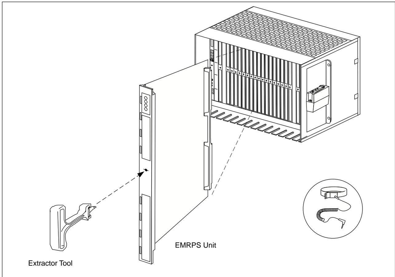
Figure 6-9. EMRPS Unit Removal
