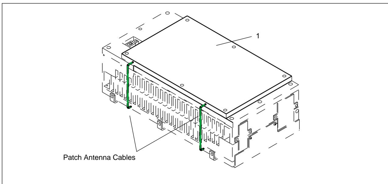
Figure B-5. Radio Head Patch Antenna Kit
