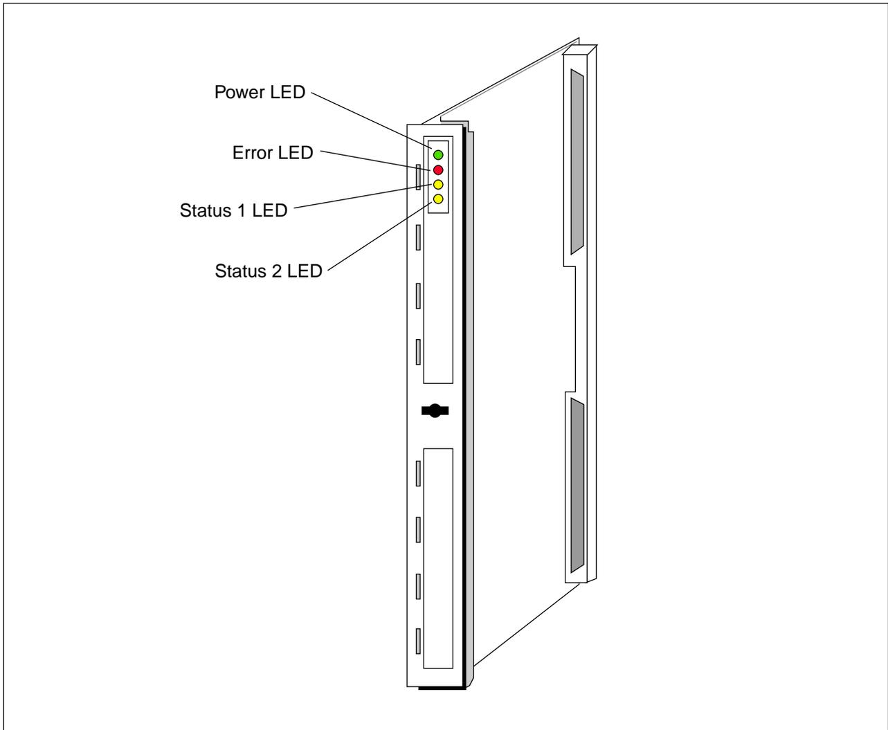
Figure 7-5. EMRPS Unit LEDs
