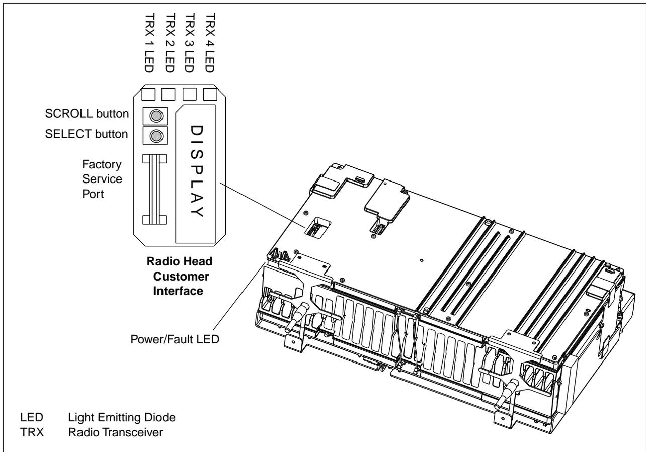
Figure 7-7. Radio Head LEDs and Customer Interface
