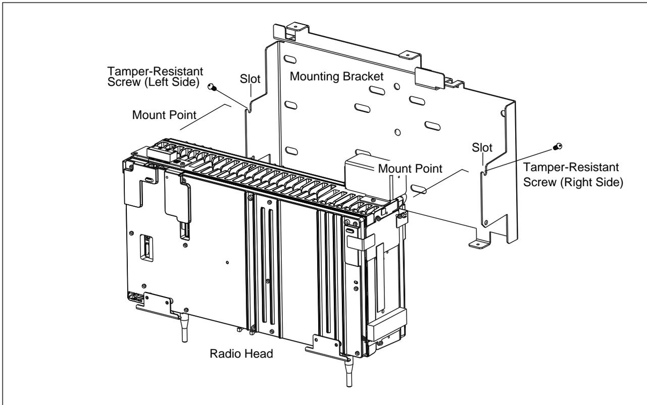
Figure 6-19. Attaching Radio Head to Mounting Bracket
