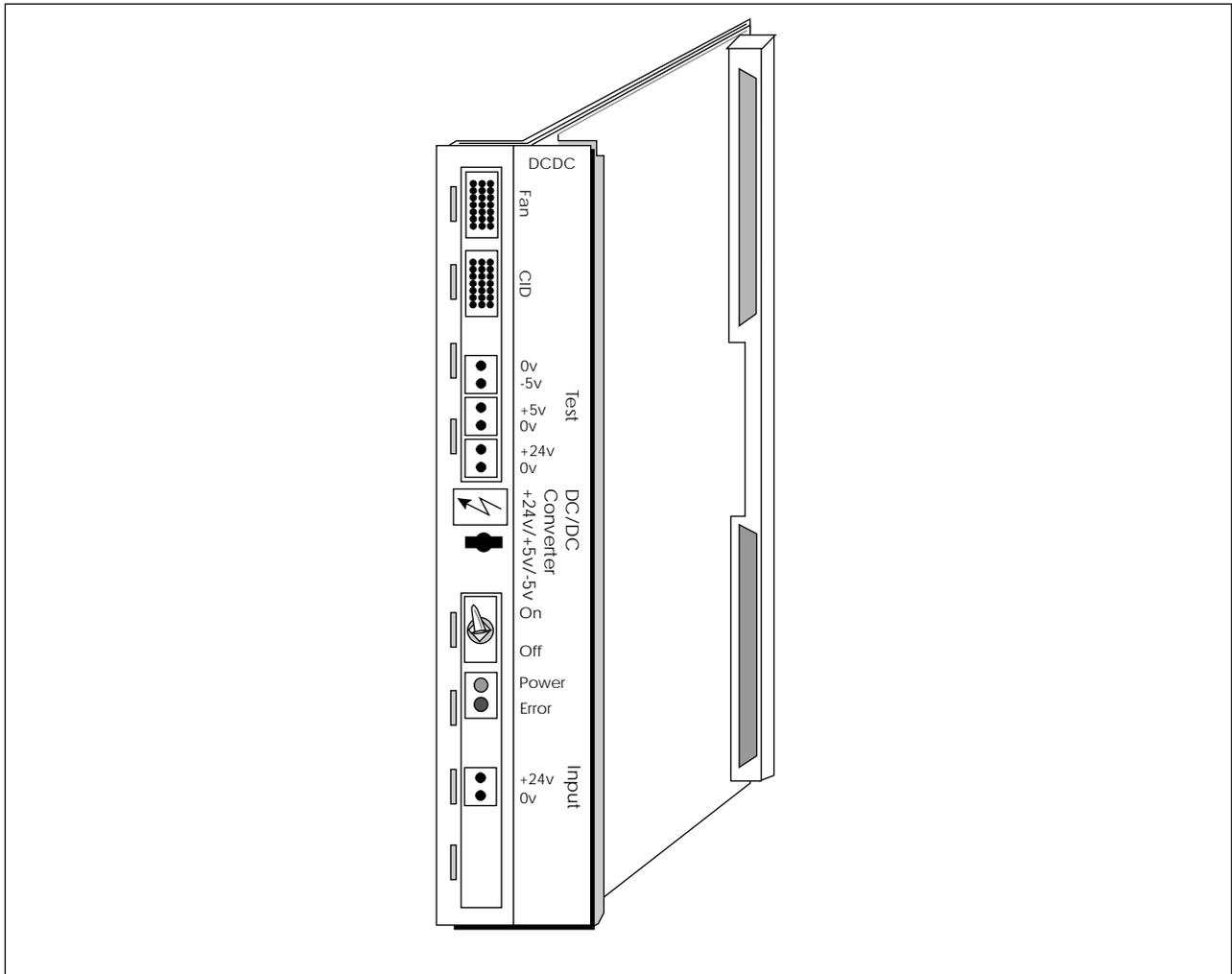
Figure 7-4. DC/DC Converter Unit LEDs
