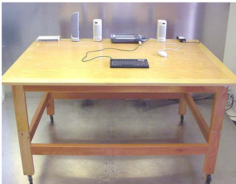
Photograph G-2 - AC Powerline Conducted Emission Configuration
