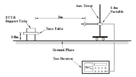
The radiated emission tests were performed in the 3-meter chamber test site, using the setup accordance with the ANSI C63.10-2013. The specification used was the FCC limits.
