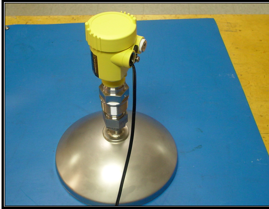
Photograph 36: EUT with 33 dBi Parabolic Antenna
