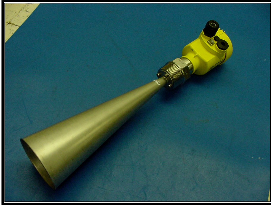
Photograph 34: EUT with 24.7 dBi Horn Antenna
