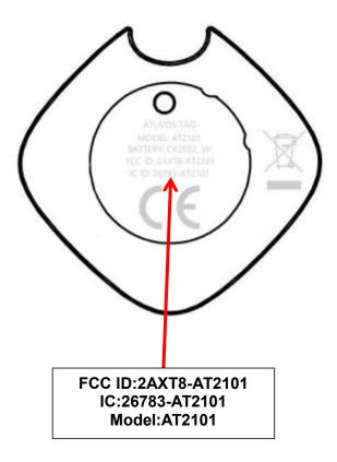
The label is etched on the rear side exterior of the device and it is always visible without using any tool.
