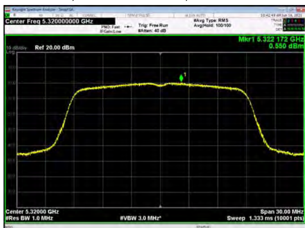
U-NII-2A, 802.11ac VHT80, Channel No.: 58
