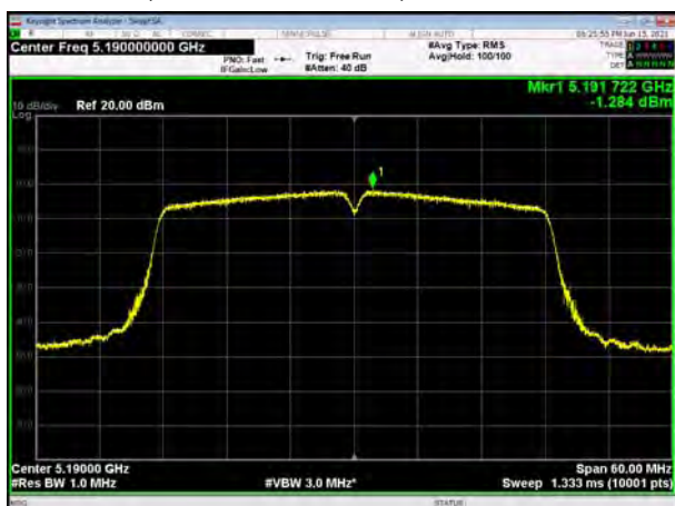
U-NII-1, 802.11ac VHT40, Channel No.: 38
