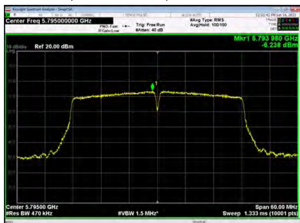
U-NII-3, 802.11ac VHT40, Channel No.: 151
