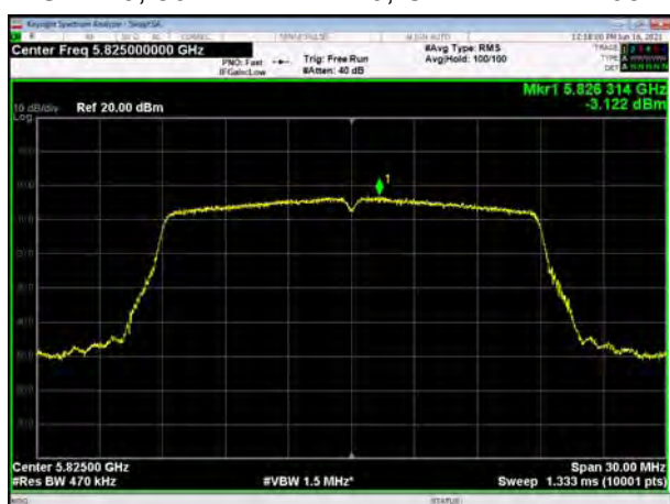
U-NII-3, 802.11ac VHT80, Channel No.: 155
