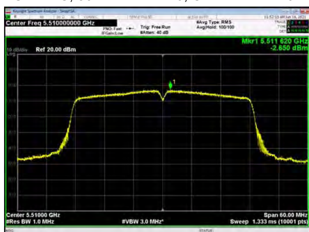
U-NII-2C, 802.11ac VHT40, Channel No.: 118
