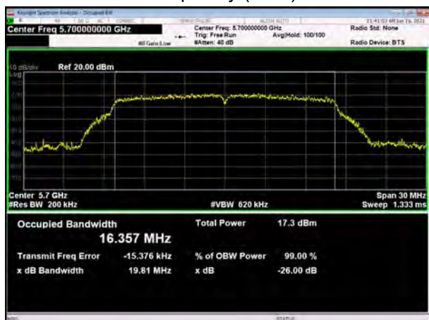
U-NII-2C, 802.11a Carrier frequency (MHz):5720
