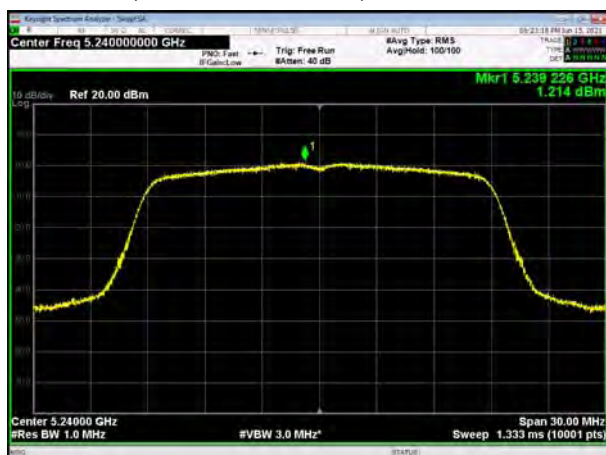
U-NII-1, 802.11ac VHT20, Channel No.: 48
