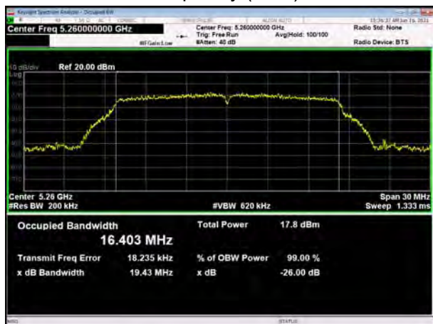
U-NII-2A, 802.11a Carrier frequency (MHz): 5300
