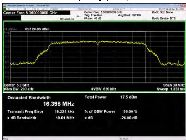
U-NII-2A, 802.11a Carrier frequency (MHz): 5300
