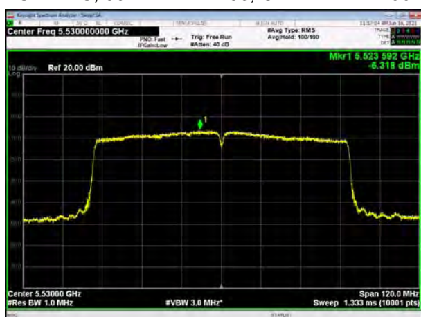
U-NII-2C, 802.11ac VHT80, Channel No.: 122
