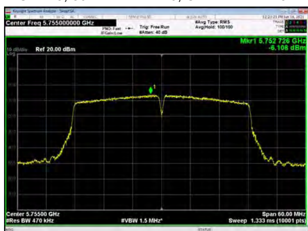
U-NII-3, 802.11ac VHT40, Channel No.: 159
