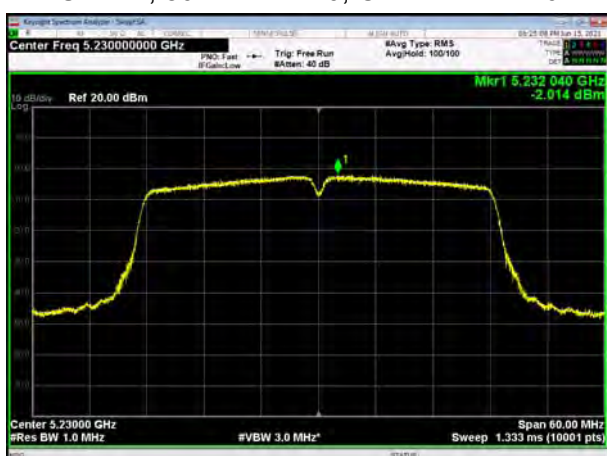
U-NII-1, 802.11ac VHT40, Channel No.: 38
