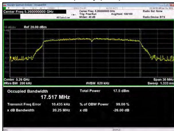
U-NII-2A, 802.11n HT20 Carrier frequency (MHz): 5300
