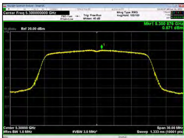
U-NII-2A, 802.11ac VHT20, Channel No.: 60
