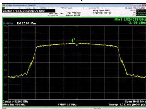
U-NII-3, 802.11ac VHT20, Channel No.: 149
