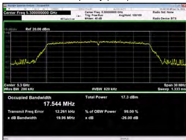
U-NII-2A, 802.11n HT20 Carrier frequency (MHz): 5300
