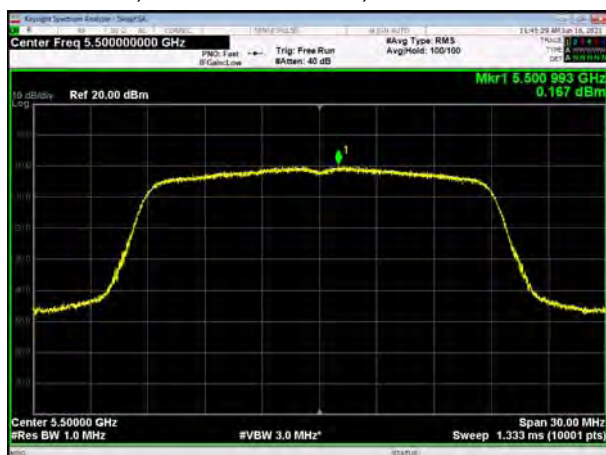
U-NII-2C, 802.11ac VHT20, Channel No.: 120
