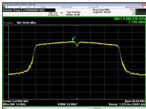
U-NII-2A, 802.11ac VHT40, Channel No.: 62
