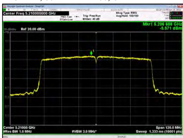
U-NII-1, 802.11ac VHT80, Channel No.: 42
