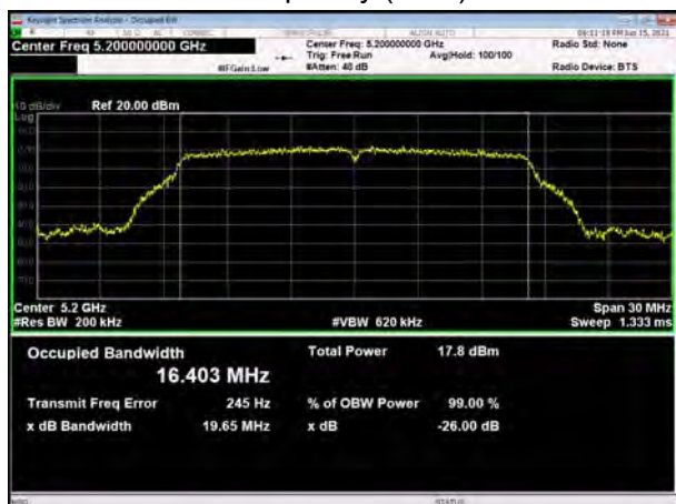
U-NII-1, 802.11a Carrier frequency (MHz): 5240
