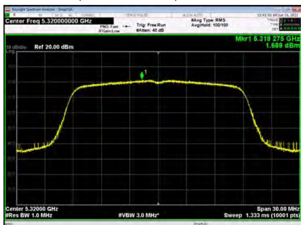
U-NII-2A, 802.11ac VHT20, Channel No.:52
