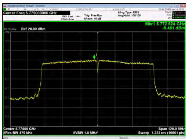
U-NII-3, 802.11ac VHT80, Channel No.: 155
