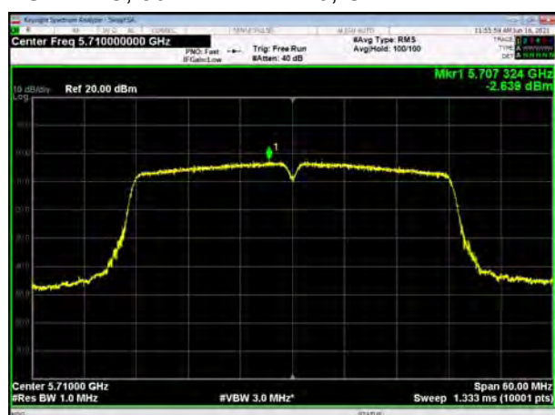
U-NII-2C, 802.11ac VHT40, Channel No.: 142
