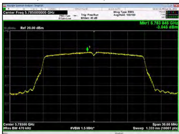
U-NII-3, 802.11ac VHT20, Channel No.: 165
