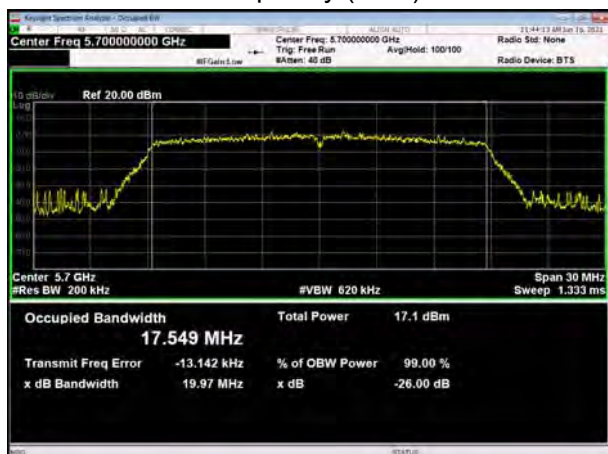
U-NII-2C, 802.11n HT20 Carrier frequency (MHz):5720
