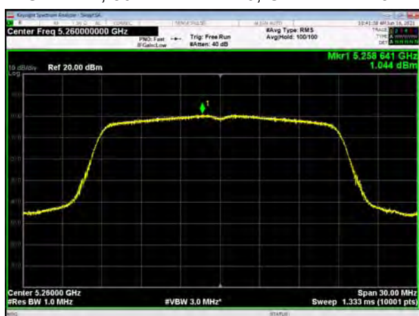
U-NII-2A, 802.11ac VHT20, Channel No.: 60
