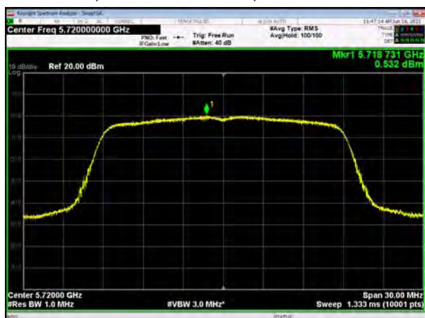
U-NII-2C, 802.11ac VHT80, Channel No.: 106
