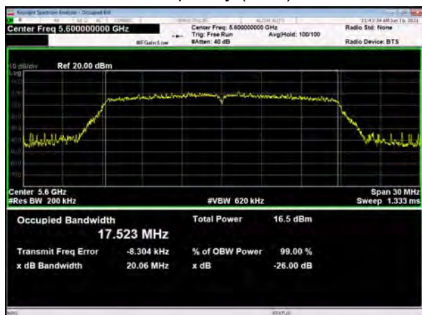
U-NII-2C, 802.11n HT20 Carrier frequency (MHz): 5700
