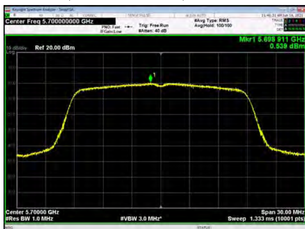
U-NII-2C, 802.11ac VHT20, Channel No.: 140
