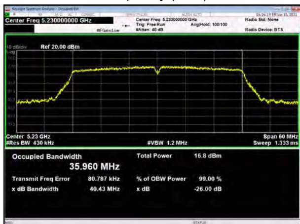
U-NII-1, 802.11ac VHT40 Carrier frequency (MHz): 5230
