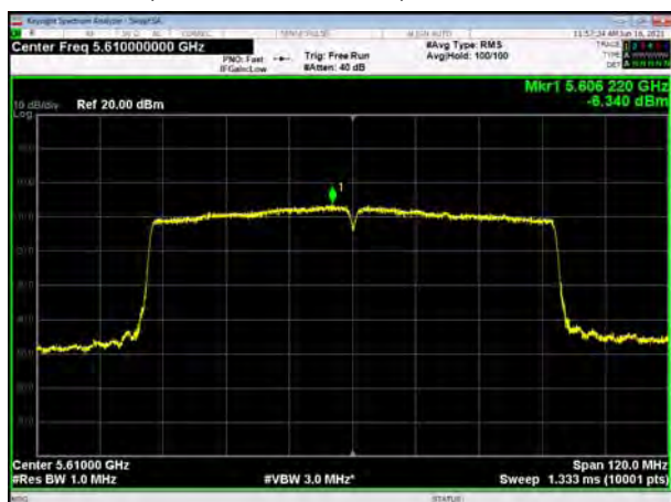
U-NII-2C, 802.11ac VHT80, Channel No.: 122
