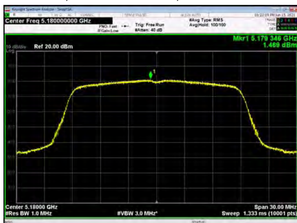
U-NII-1, 802.11ac VHT20, Channel No.: 40
