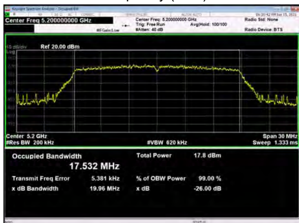
U-NII-1, 802.11n HT20 Carrier frequency (MHz): 5240
