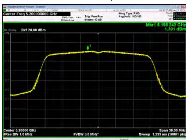
U-NII-1, 802.11ac VHT20, Channel No.: 48
