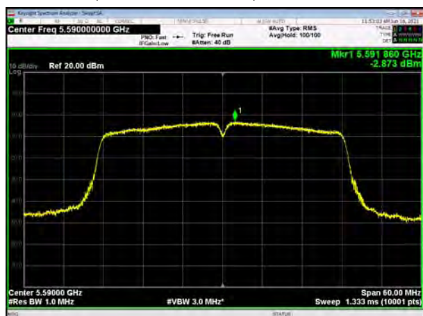
U-NII-2C, 802.11ac VHT40, Channel No.: 118
