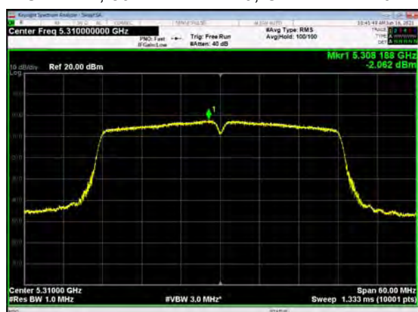
U-NII-2A, 802.11ac VHT40, Channel No.: 62
