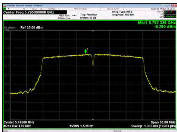
U-NII-3, 802.11ac VHT40, Channel No.: 159
