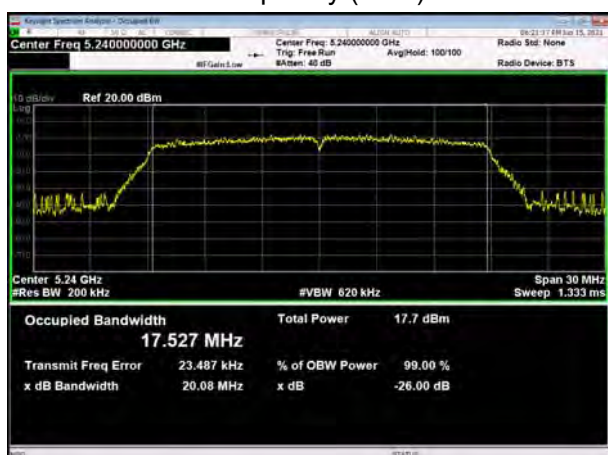
U-NII-1, 802.11n HT20 Carrier frequency (MHz): 5240
