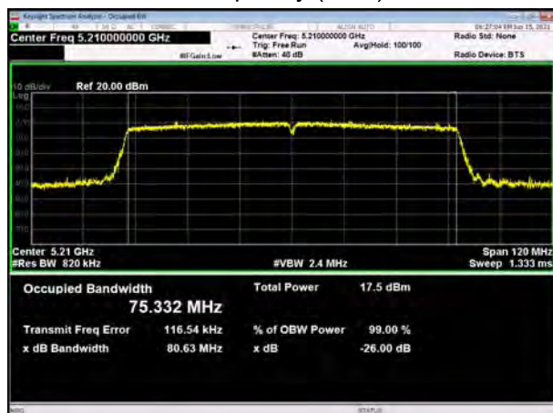
U-NII-1, 802.11ac VHT80 Carrier frequency (MHz): 5210
