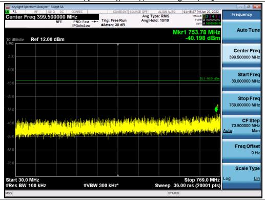
Antenna 0 / Low Edge - 100 MHz ~ Low Edge / (2 Port)B5 LTE B5 5 MHz 1 Carrier + (5G NR n5 5 MHz 1 Carrier + B5 DSS 10 MHz 1 Carrier) [3 Carrier](1C+2C) / Non-Contiguous / 256QAM
