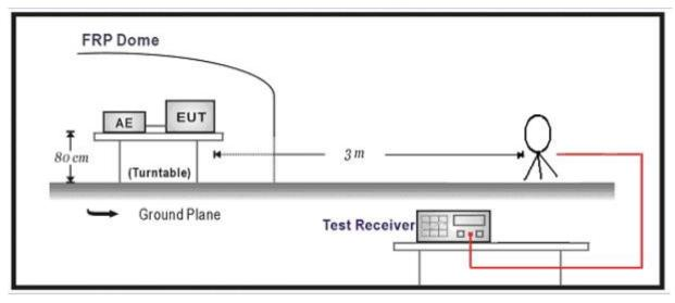
Below 1GHz Test Setup:
