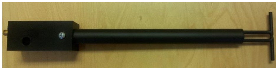
Figure 1 – MVG COMOSAR Validation Dipole
