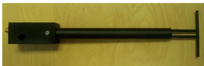
Figure 1 – MVG COMOSAR Validation Dipole
