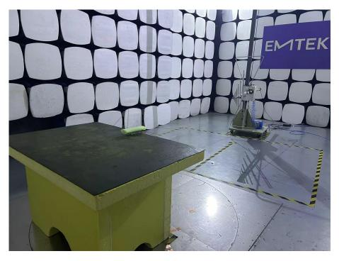
Spurious Emission Test Setup (Above 1GHz)
