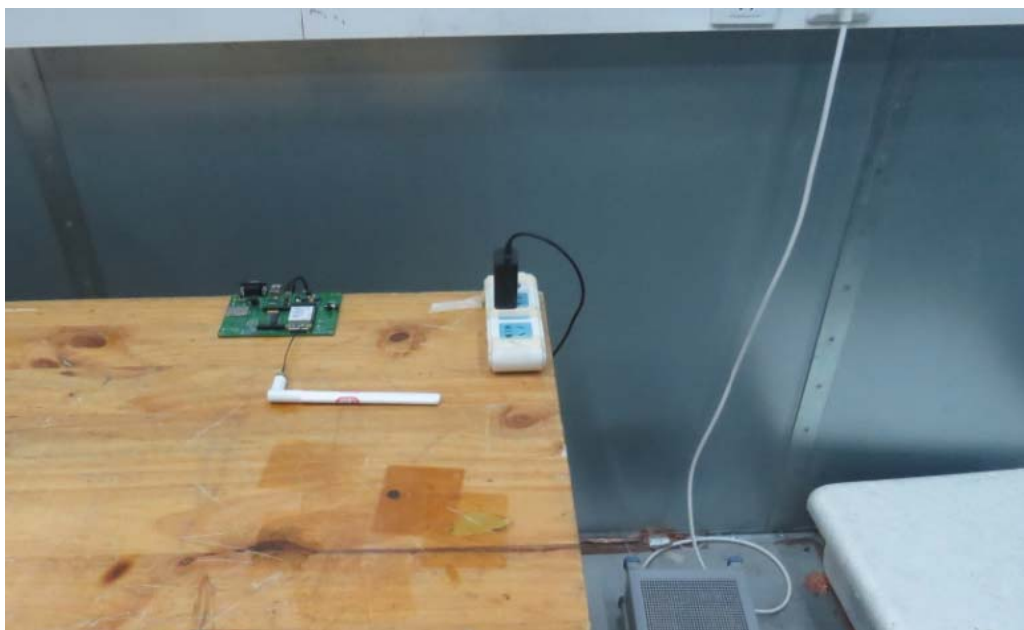
Picture 2 Conducted Emission Test Setup
