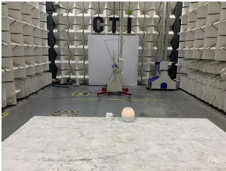
Radiated spurious emission Test Setup-1(Below 1GHz)
