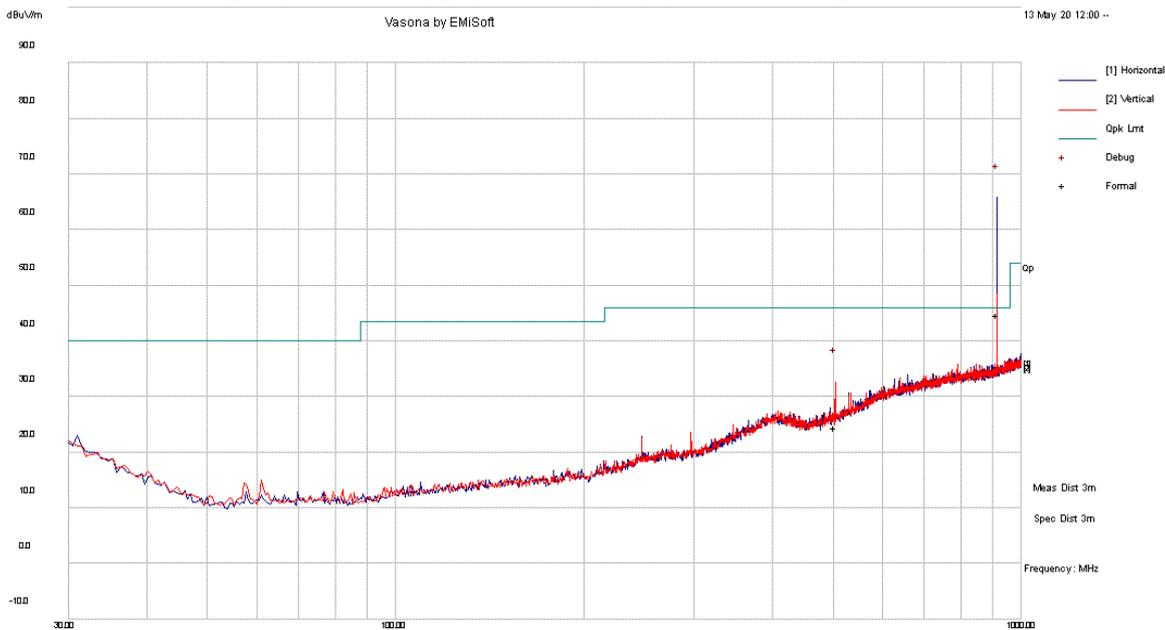
Radiated Emissions      Template: FCC Class B (3m) 30MHz-1GHz
