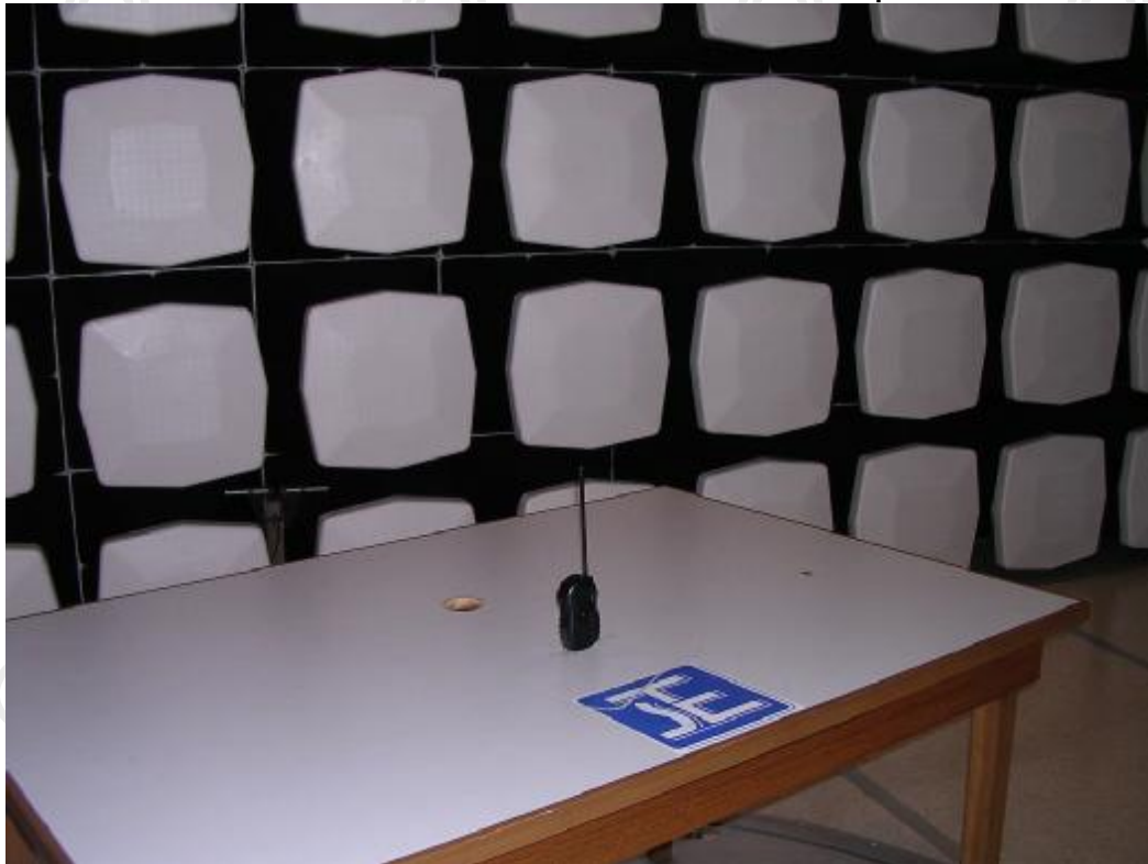
Measurement of Radiated Emission Test Set Up
