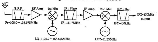
The first frequency converter circuit (1st MIX) mixes the received signal with the first local oscillator signal, whose frequency (LO1) is higher than the selected receive frequency (Fr) by the first intermediate frequency (IF1: 21.7 MHz), to down-convert the received signal to the first intermediate frequency band (Fr to IF1).
