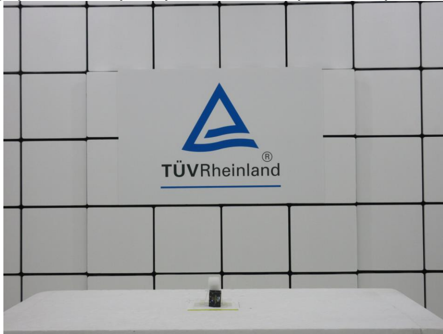
Photograph 1: Test Setup for Spurious Emissions (Front View 1)
