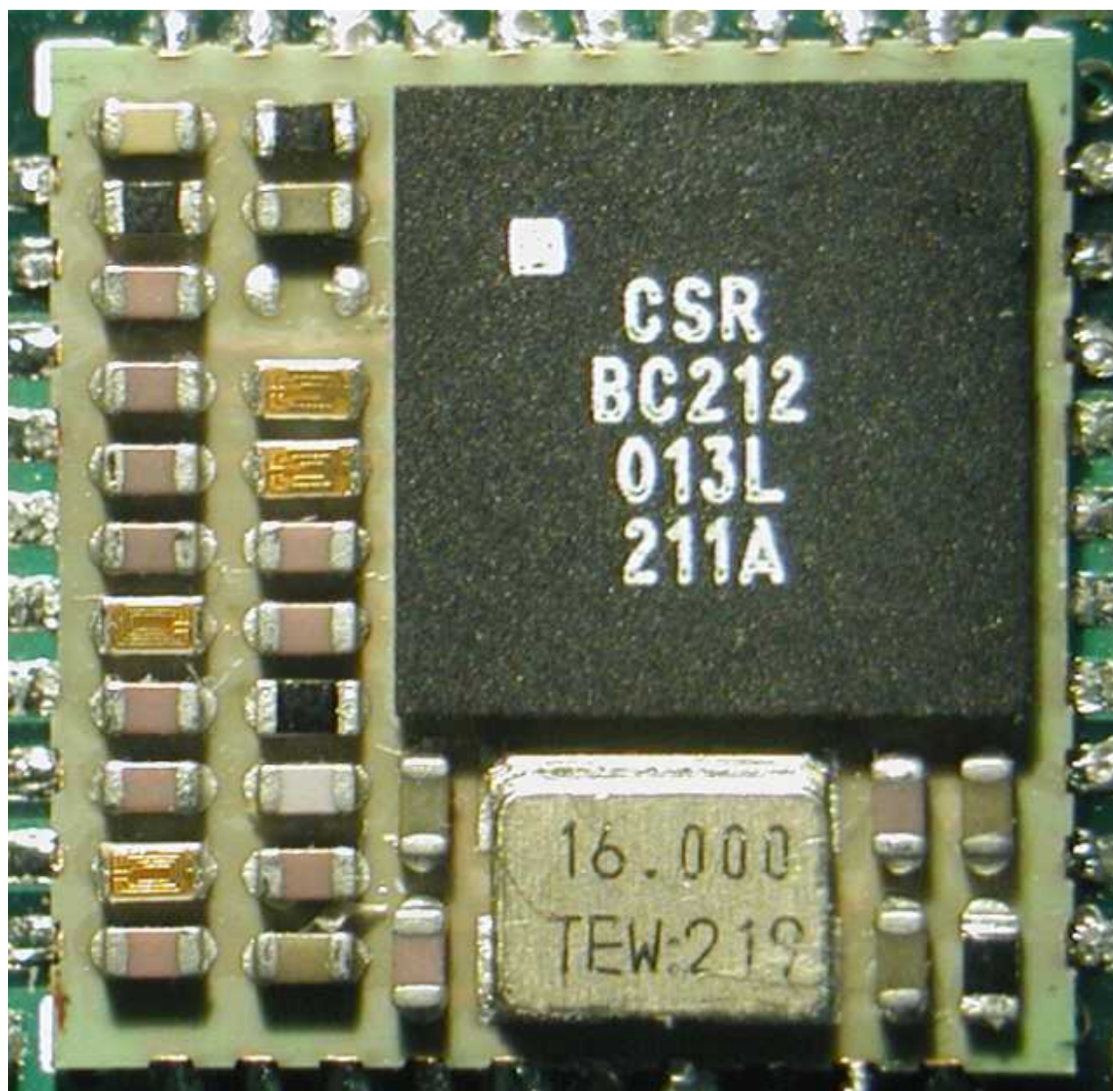
Radio Module – Internal View
