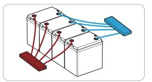
0 Bus Bar: It can help ensure the input & output currents of each battery are balanced and improve the conversion efficiency of the input & output currents for the battery.
