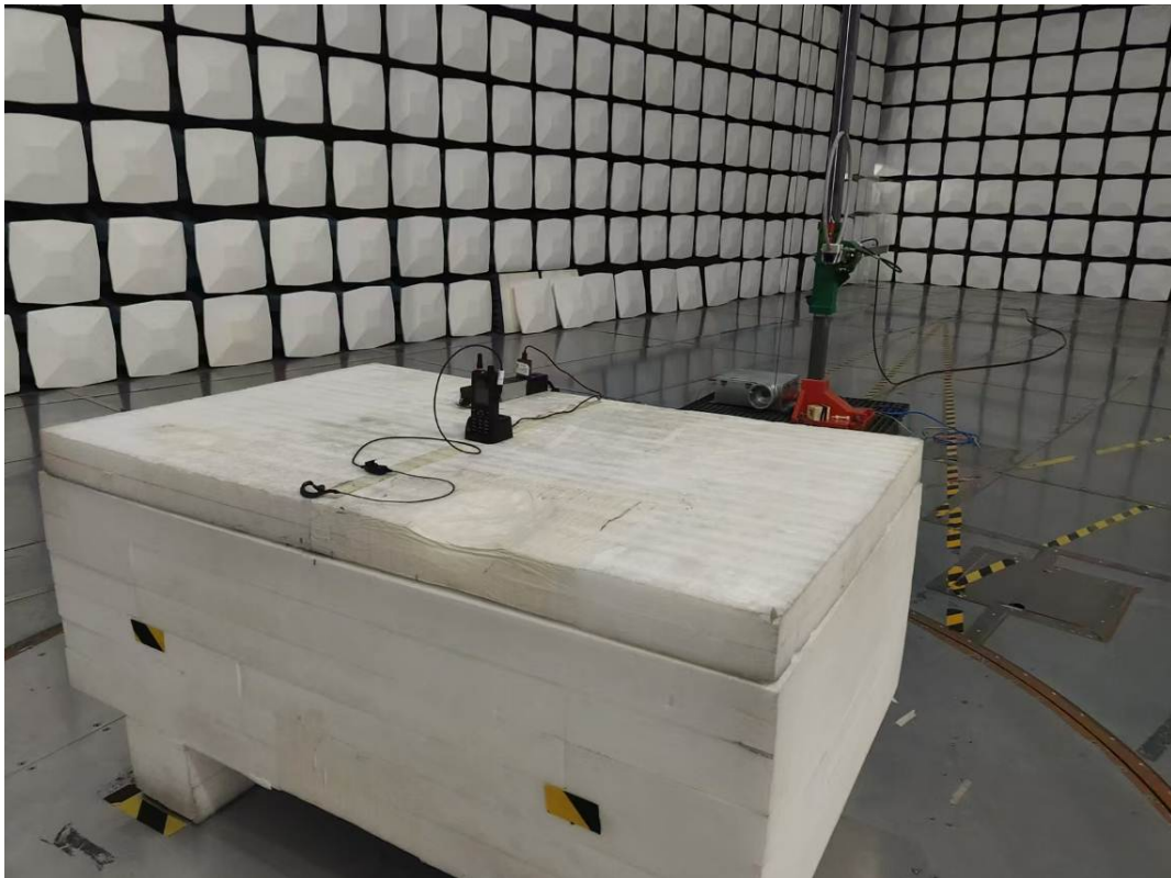
Radiated Emission 9k-30MHz Perpendicular View
