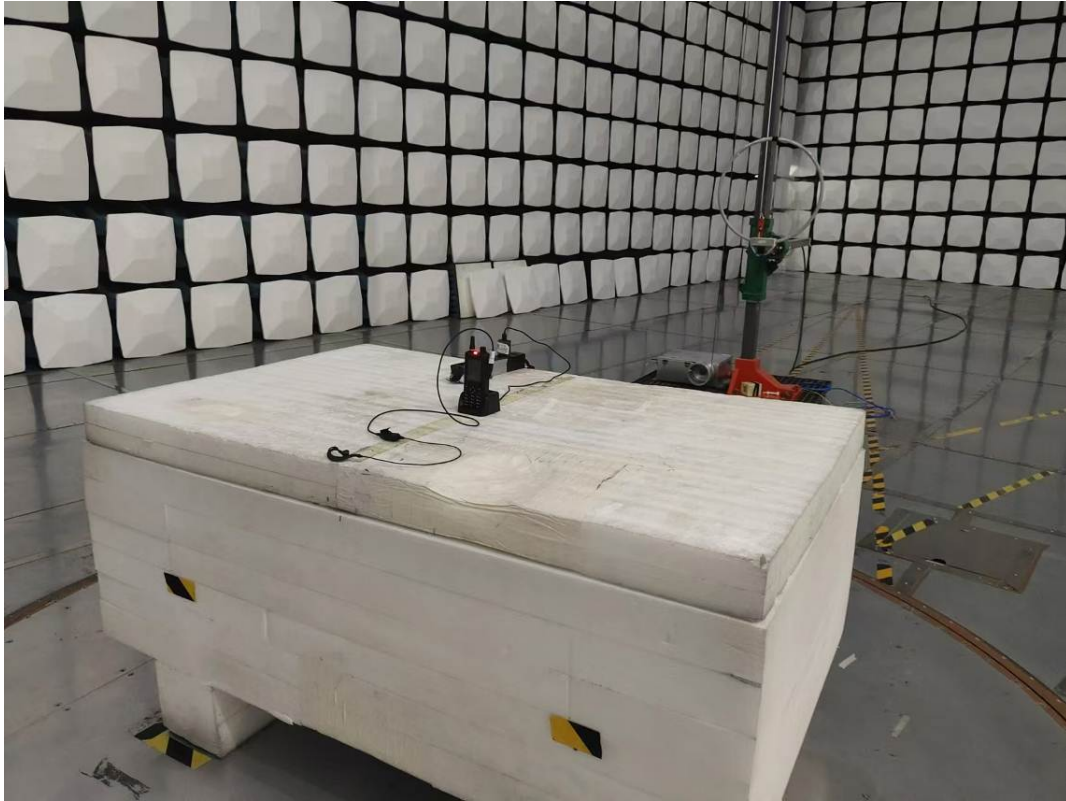
Radiated Emission 9k-30MHz Perpendicular View
