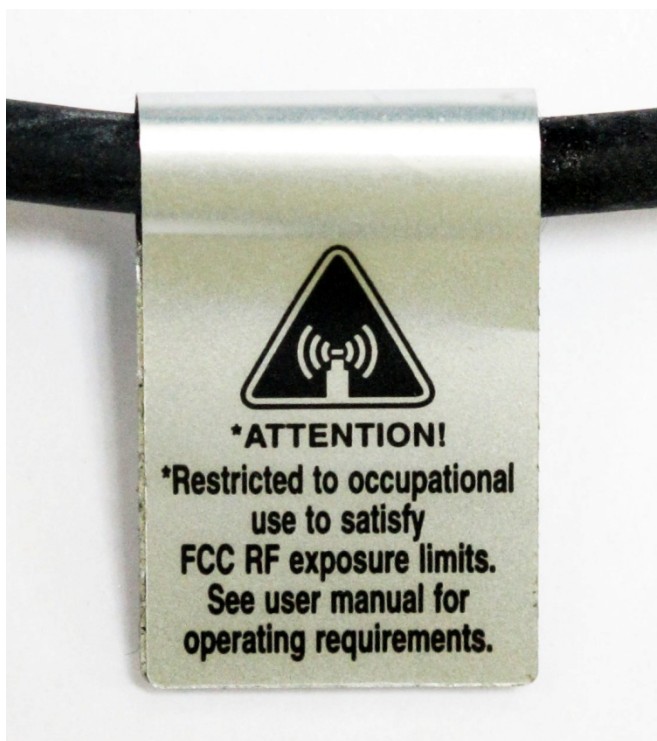
RF Exposure Label (Close View)
