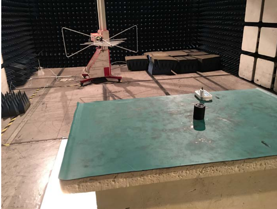
Spurious Emission Test Setup (Below 1GHz)
