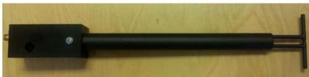
Figure 1 – MVG COMOSAR Validation Dipole
