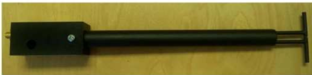
Figure 1 – MVG COMOSAR Validation Dipole
