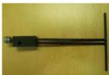
Figure 1 – MVG COMOSAR Validation Dipole
