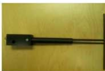
Figure 1 – MVG COMOSAR Validation Dipole
