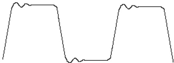
Caution: If modulation balance is not tuned properly like following pictures, it causes error in TX sub-tone modulation.
