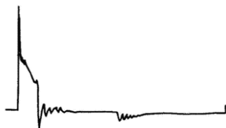
Secondary circuit resistance is too large
