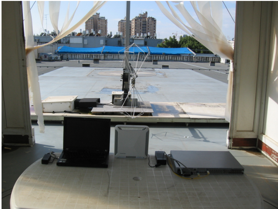
Radiated Emission Test, 30-200MHz
