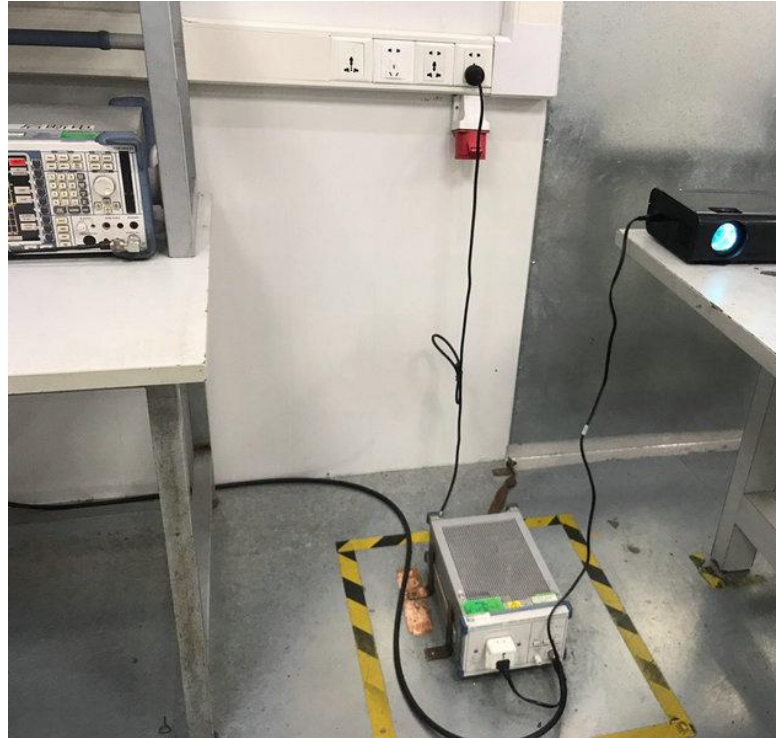
Photo of Power Line Conducted Emission Test
