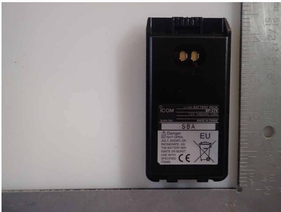
Li-ion Chargeable Battery (M/N: BP-279, 7.2V, 1485mAh)
