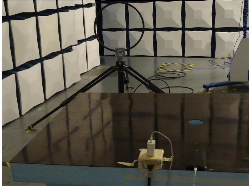
Radiated Disturbance Emissions (9Khz-30Mhz)
