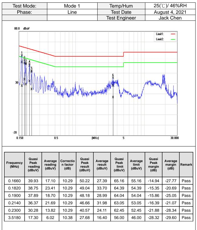
Note: Correction factor = LISN loss + Cable loss.
