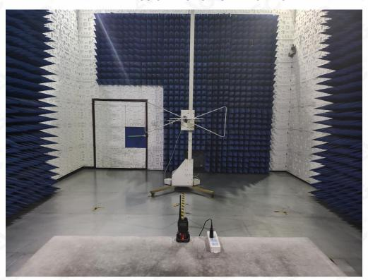
RADIATED EMISSION TEST SETUP ABOVE 1GHz
