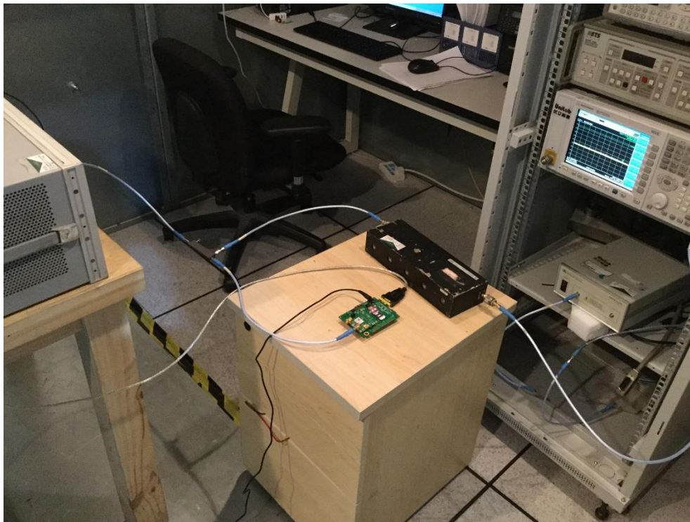
Frequency Stability Under Temperature & Voltage Variations Setup
