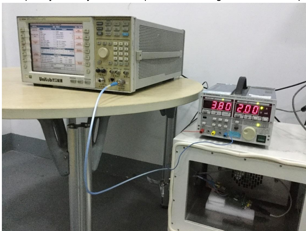
Frequency Stability Under Temperature & Voltage Variations Setup
