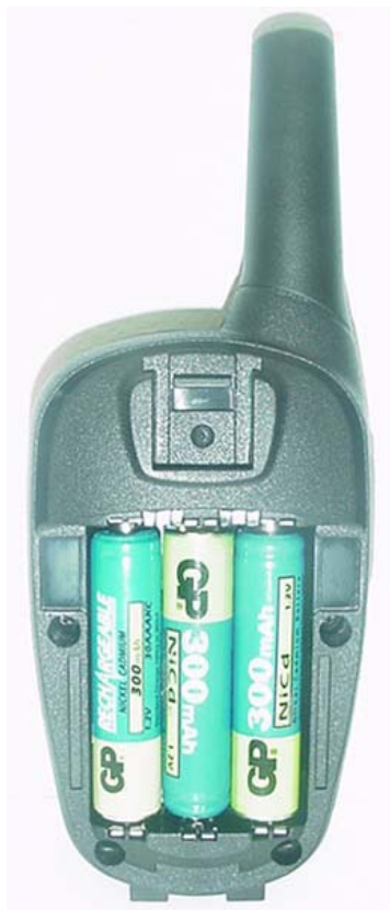
DUT with NiCd AAA Batteries
