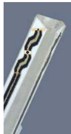
ET3DV6 E-Field Probe
