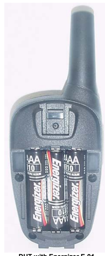
DUT with Energizer E-91 AAA Alkaline Batteries
