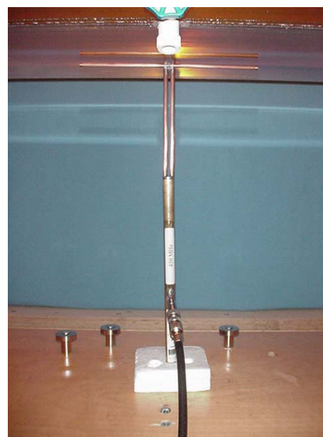
450 MHz Dipole Setup
