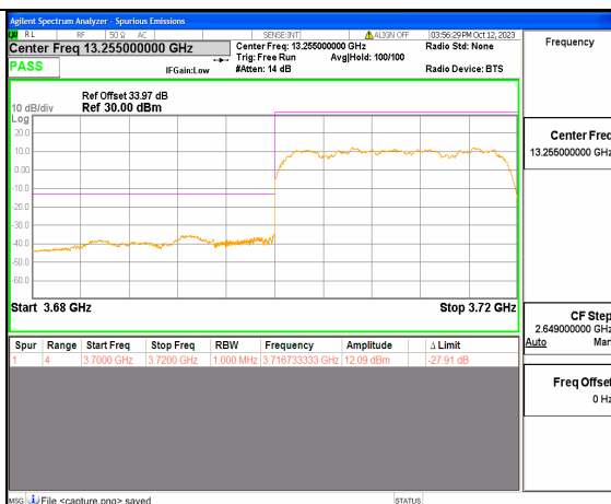
5A_n77(3700-3980MHz) 20M DFT-s-OFDM QPSK Outer_Full Low
