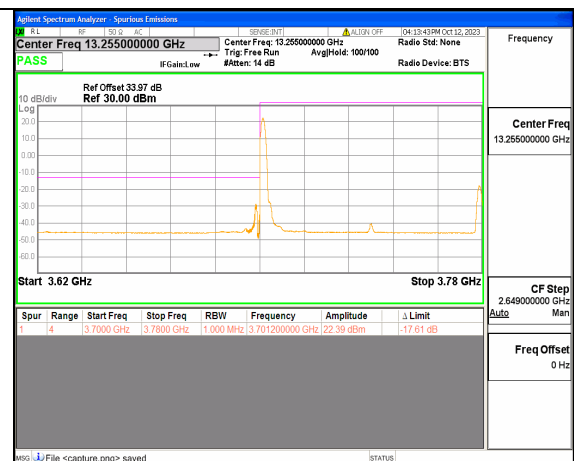
5A_n77(3700-3980MHz) 80M DFT-s-OFDM QPSK Edge_1RB_Left Low
