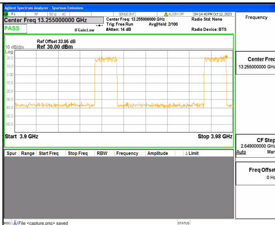
5A_n77(3700-3980MHz) 80M DFT-s-OFDM QPSK Outer_Full High
