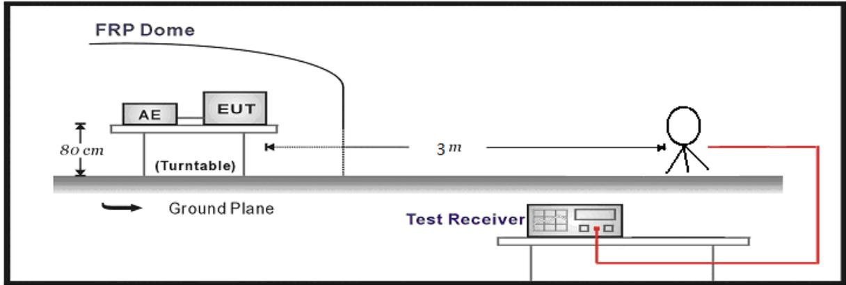
Below 1GHz Test Setup:
