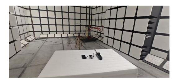
Radiated Emissions View (30 MHz- 1 GHz) -antenna 1&2
