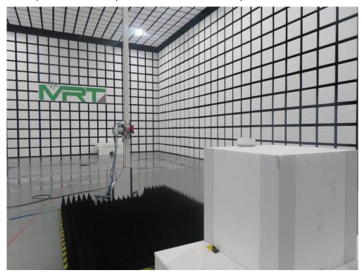
Description: Radiated Spurious Emission Test Setup for Above 18GHz
