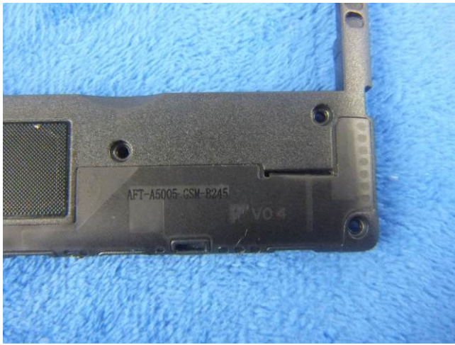
GSM/PCS/UMTS-FDD Antenna View
