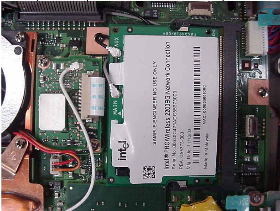
Calexico2 (WM3B2200BG) WLAN & Bluetooth – UGXZ5-102A – exploded view
