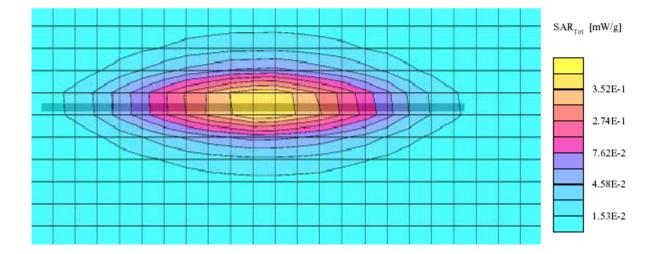
300 MHz Head Liquid System Validation (Ambient Temp = 23 Deg C, Liquid Temp = 22 Deg C, Forward Power = 20.12 dBm, 01/03/2005)
