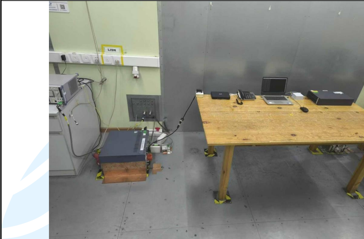
Conducted Emission Test Setup
