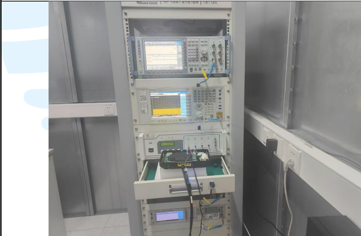
RF Conducted Test Setup
