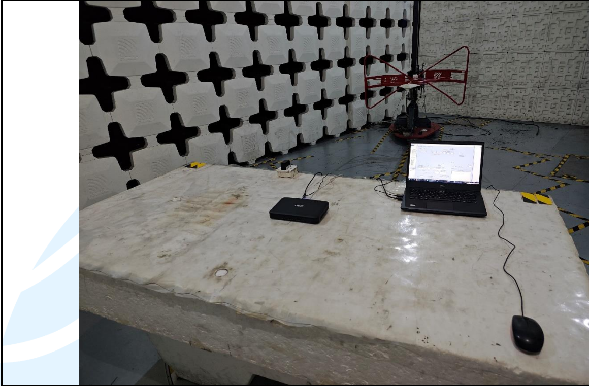
Radiated emission Test Setup (30 MHz~1 GHz)
