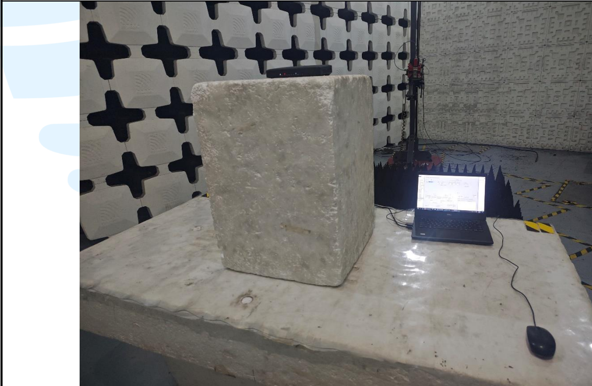
Radiated emission Test Setup (Above 1 GHz)
