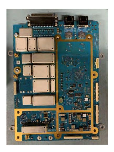
Internal Front View - Modem Module Bottom View - Heat Sink Removed
