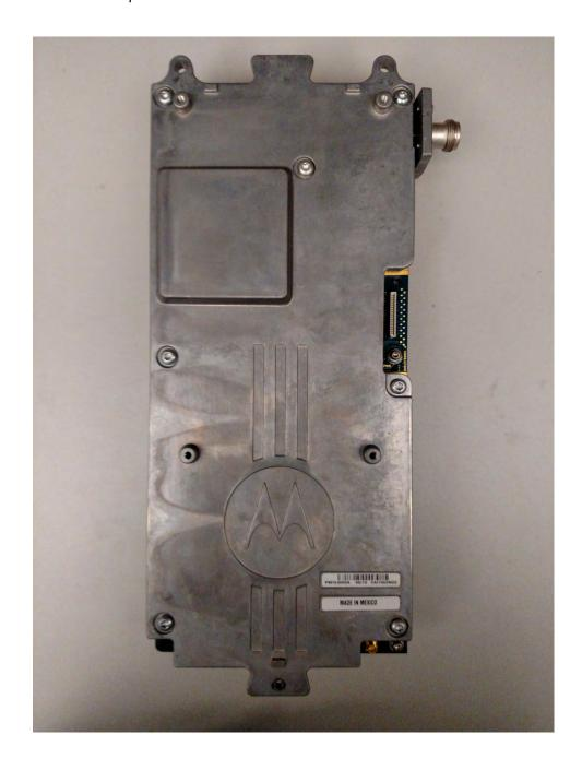
Internal Front View – Power Amplifier Module – Top View, Cover Removed
