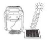
Connect The Solar Panel To Your Device Using The Multi Head USB Cable.
