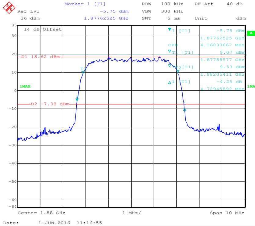
**99% Occupied Bandwidth&26 dB Bandwidth for HSUPA (BPSK) Mode**
