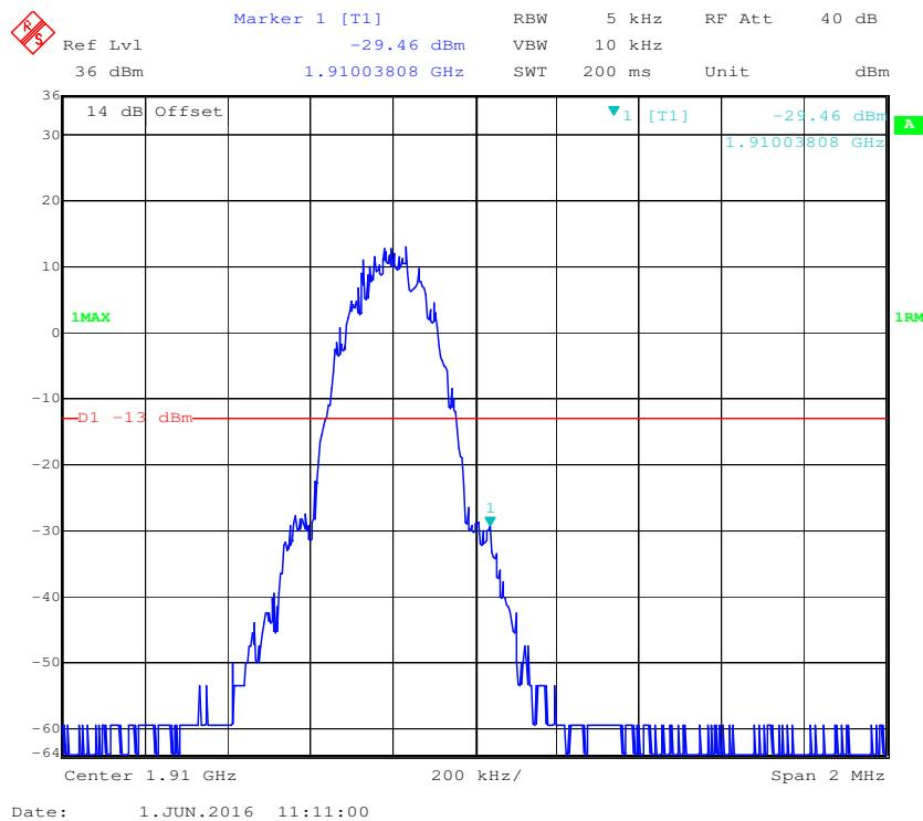
**PCS Band, Left Band Edge for RMC (BPSK) Mode**
