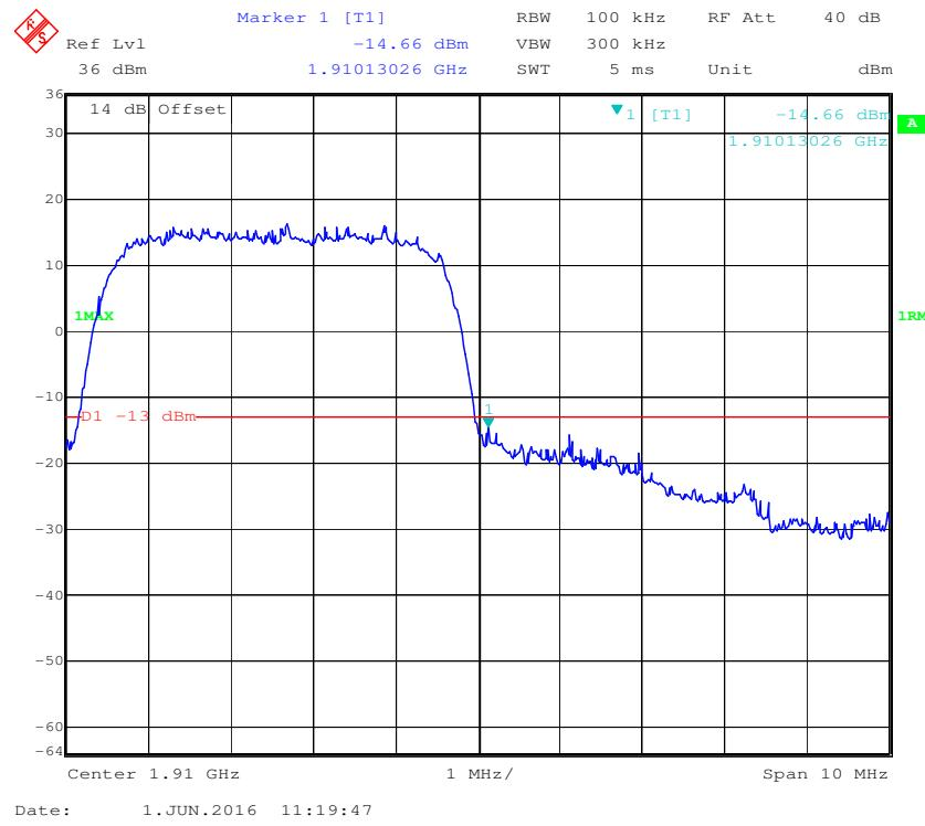
**PCS Band, Left Band Edge for HSDPA (16QAM) Mode**
