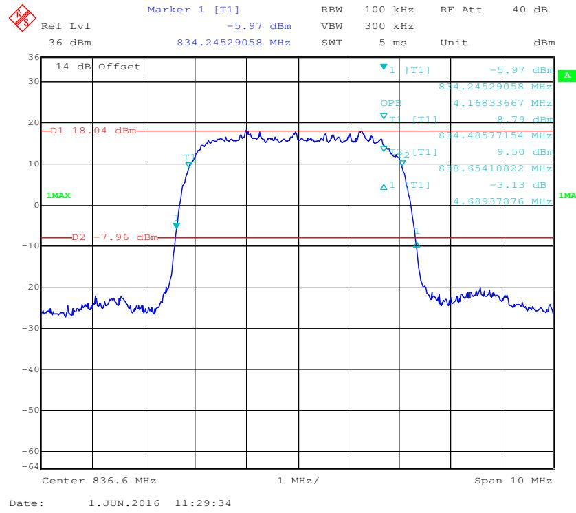
**99% Occupied Bandwidth&26 dB Bandwidth for HSUPA (BPSK) Mode**
