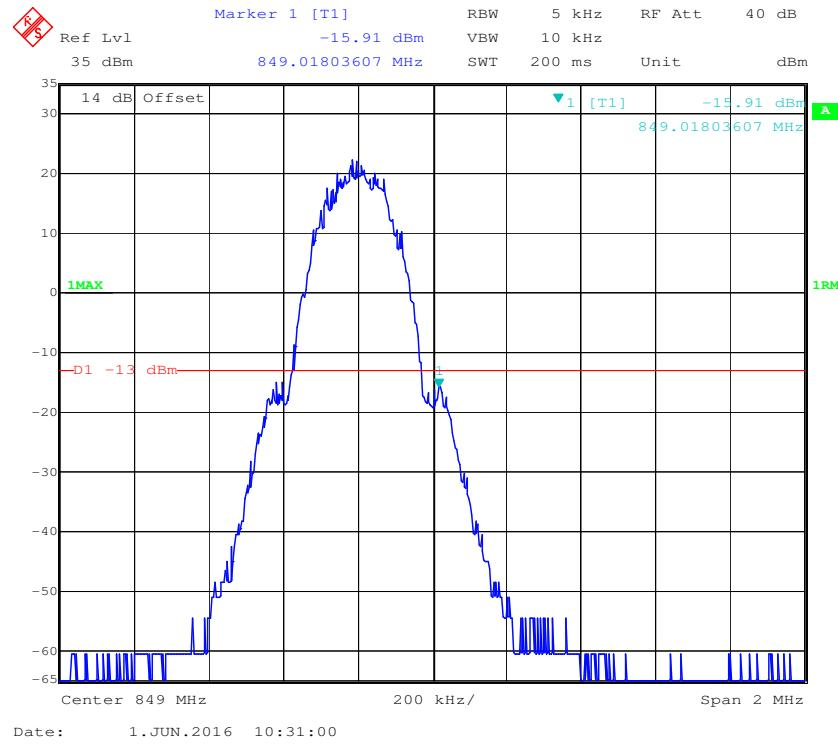
**Cellular Band, Left Band Edge for GSM (EGPRS) Mode**
