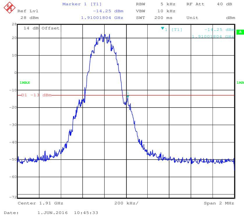
**PCS Band, Left Band Edge for GSM (EGPRS) Mode**
