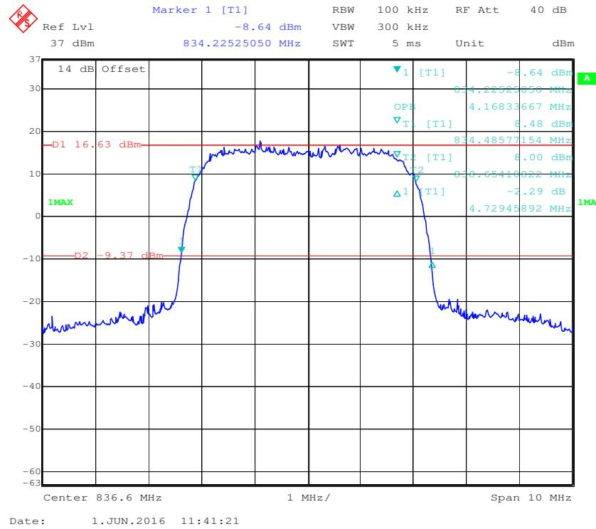
**99% Occupied Bandwidth&26 dB Bandwidth for HSDPA (16QAM) Mode**
