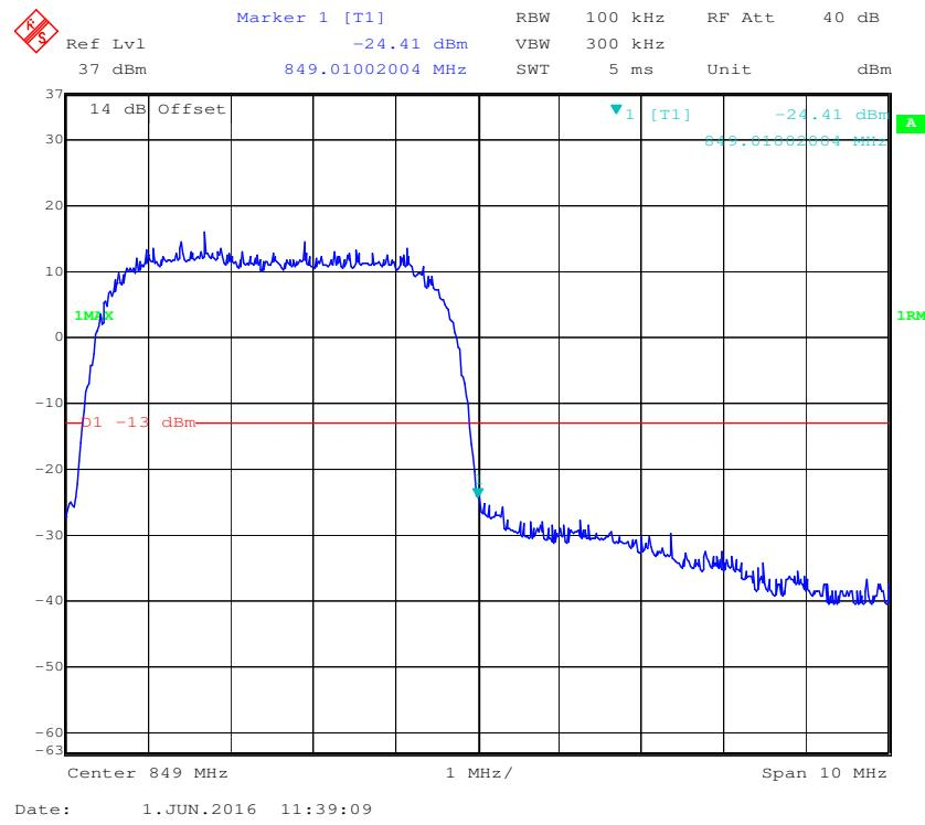
**PCS Band, Left Band Edge for GSM (GMSK) Mode**
