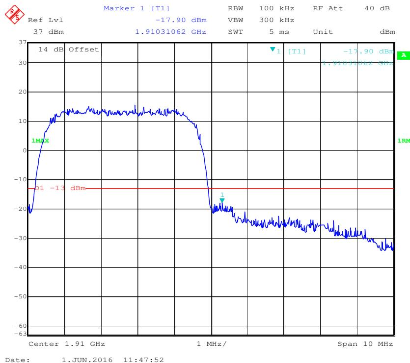
**PCS Band, Left Band Edge for HSUPA (BPSK) Mode**
