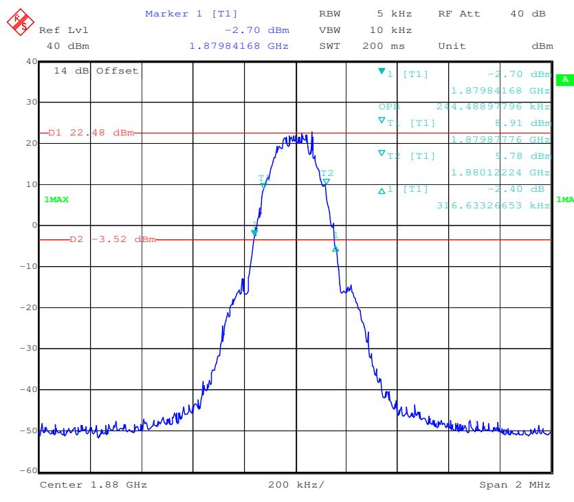
**26 dB Occupied Bandwidth for EDGE (8PSK) Mode**
