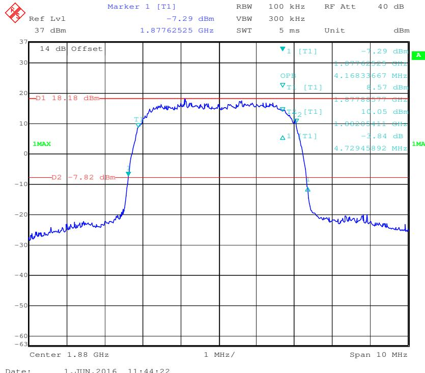
**99% Occupied Bandwidth&26 dB Bandwidth for HSDPA (16QAM) Mode**
