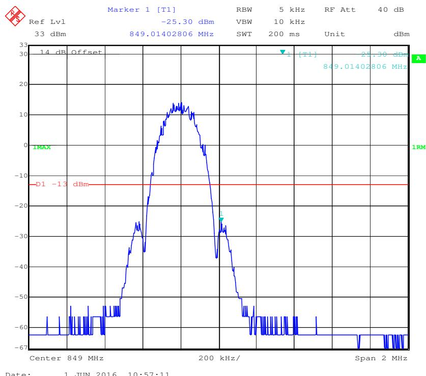
**Cellular Band, Left Band Edge for RMC (BPSK) Mode**
