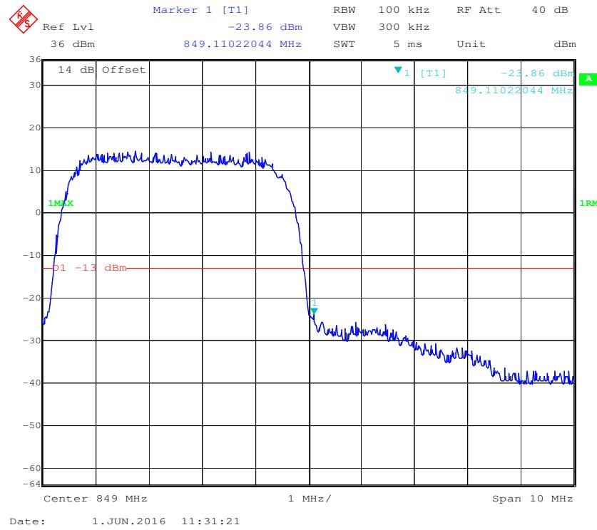
**Cellular Band, Left Band Edge for HSDPA (16QAM) Mode**
