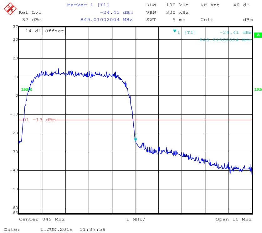
**Cellular Band, Left Band Edge for HSUPA (BPSK) Mode**
