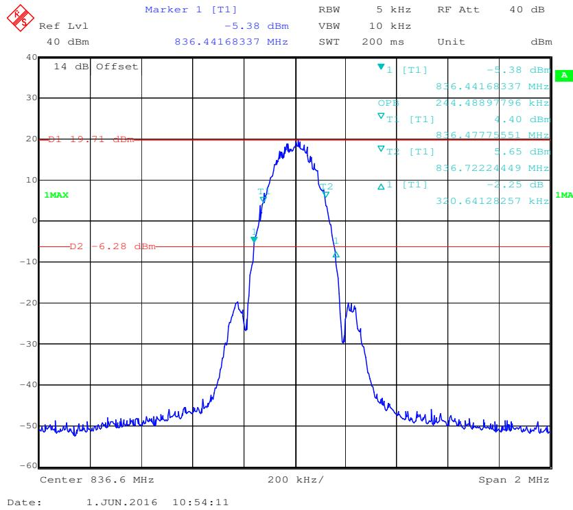
**99% Occupied Bandwidth&26 dB Bandwidth for RMC (BPSK) Mode**
