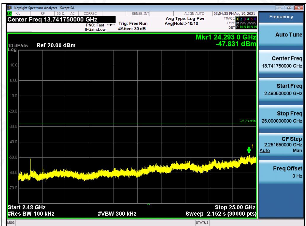
Test_Graph_EDR_ANT1_2402_3Mbps_Higher Band Emissions
